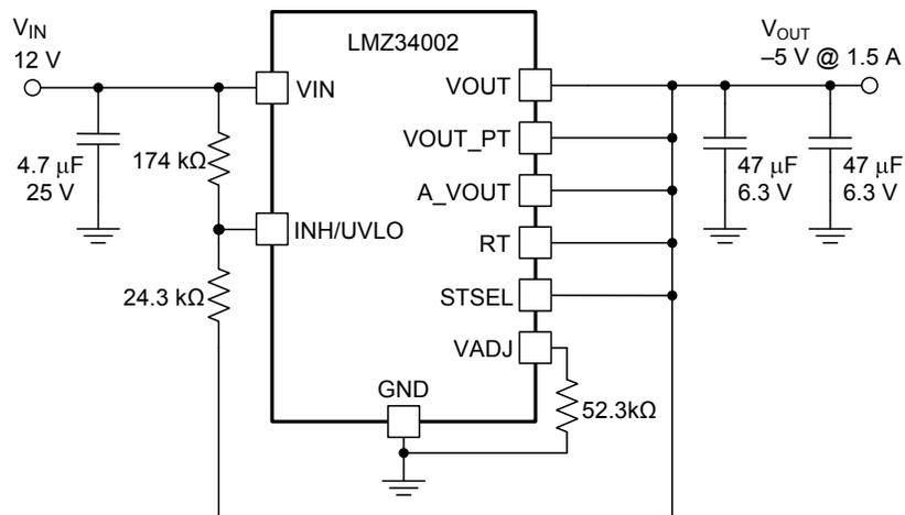
**Figure 35. Typical Schematic**
