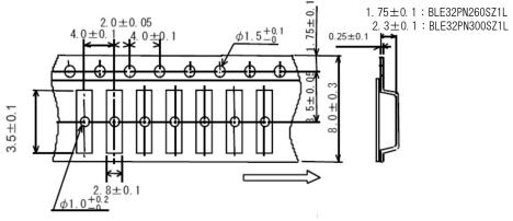
(in mm) \*Dimension of the Cavity is measured at the bottom side.
