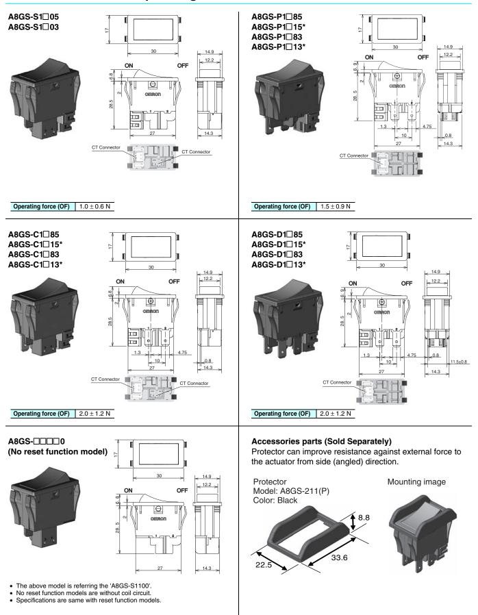
Note: 1. Unless otherwise specified, a tolerance of ± 0.4 mm applies to all dimensions.
