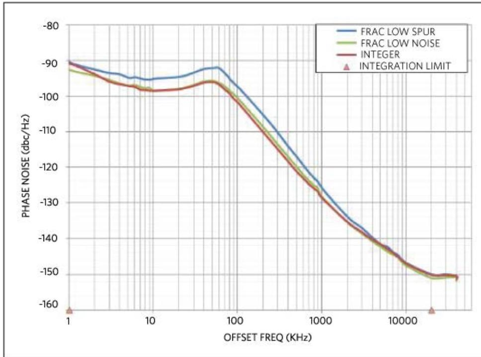
Figure 2. 12GHz phase noise plot.
