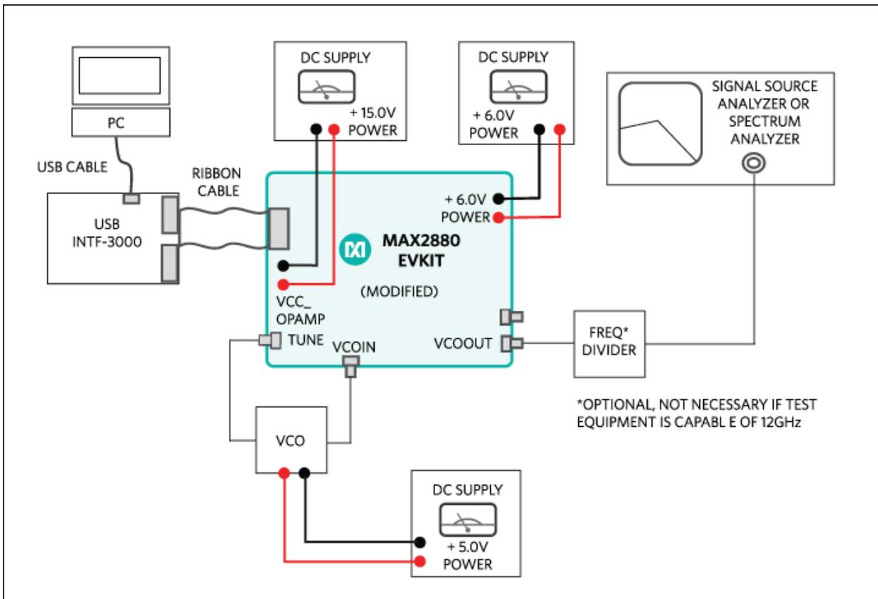
Figure 4. Detail setup diagram.
