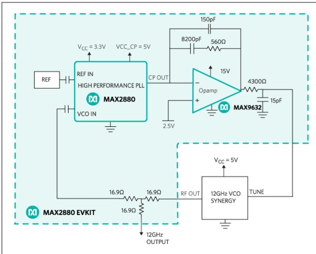
Figure 1. 12GHz ultra-low phase noise fractional-N PLL based on MAX2880.
