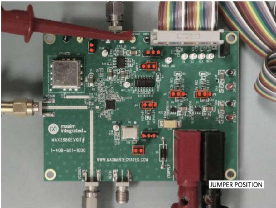
Figure 3. Jumper position.
