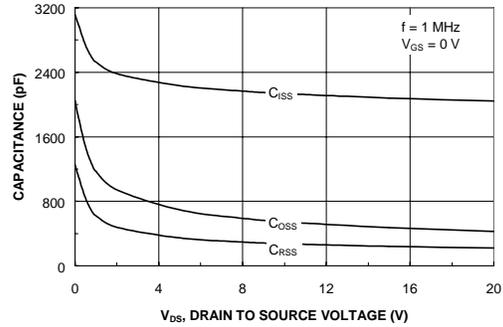
**Figure 8. Capacitance Characteristics.**
