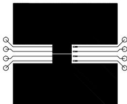
a)  $78^\circ\text{ C/W}$  when mounted on a  $0.5\text{ in}^2$  pad of 2 oz. copper.
