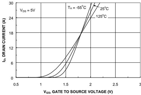
Figure 5. Transfer Characteristics.
