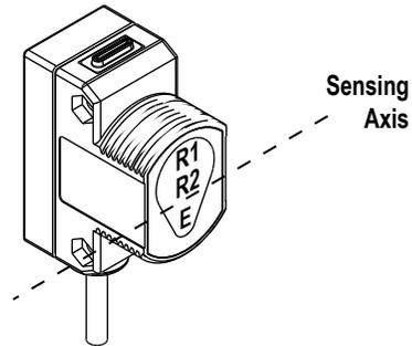
In the drawings and information provided in this document, the letters E, R1, and R2 identify how the sensor's three optical elements (Emitter "E", Near Detector "R1", and Far Detector "R2") line up across the face of the sensor. The location of these elements defines the sensing axis, see Figure 2 on p. 2. The sensing axis becomes important in certain situations, such as those illustrated in Figure 5 on p. 3 and Figure 6 on p. 3.
