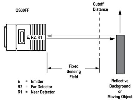
A reflective background object in this position or moving across the sensor face in this axis is ignored.
