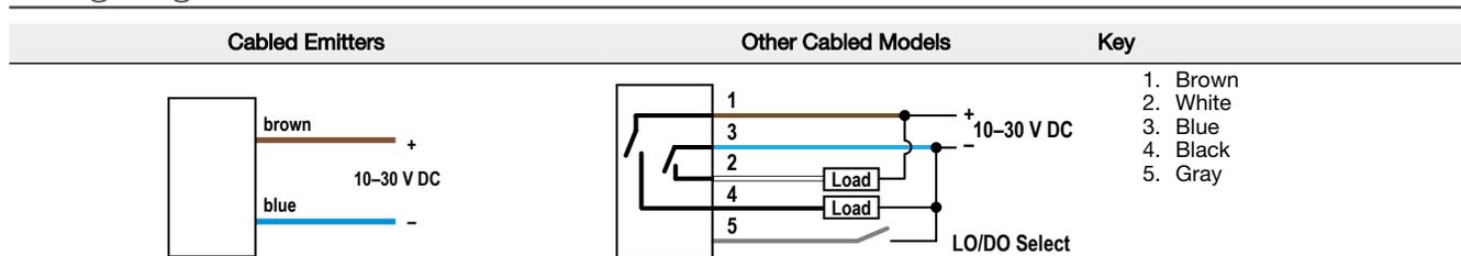
Cabled wiring diagrams are shown. Quick disconnect wiring diagrams are functionally identical.
