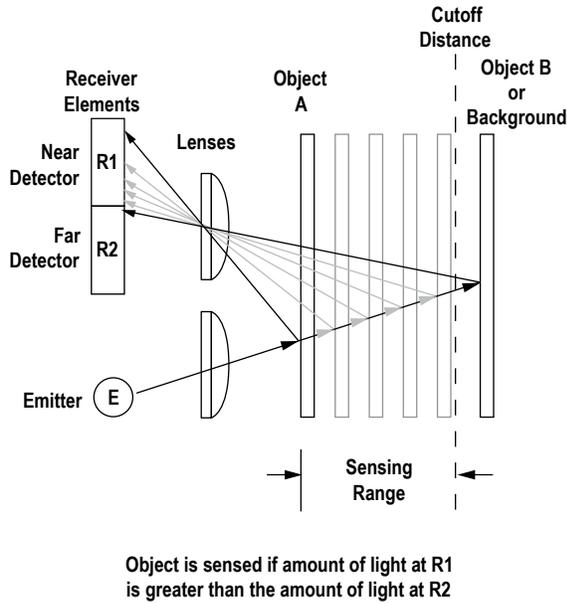
Figure 2. Fixed-Field Sensing Axis
