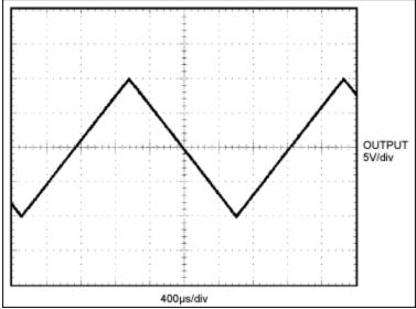
Figure 2. Voltage-follower output for a 400Hz triangle-wave input.
