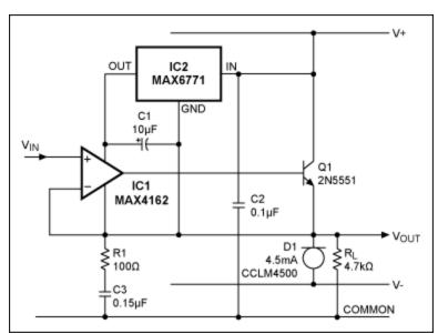
Figure 1. By leveraging a low-dropout regulator, this voltage follower can achieve an extended voltage swing.
