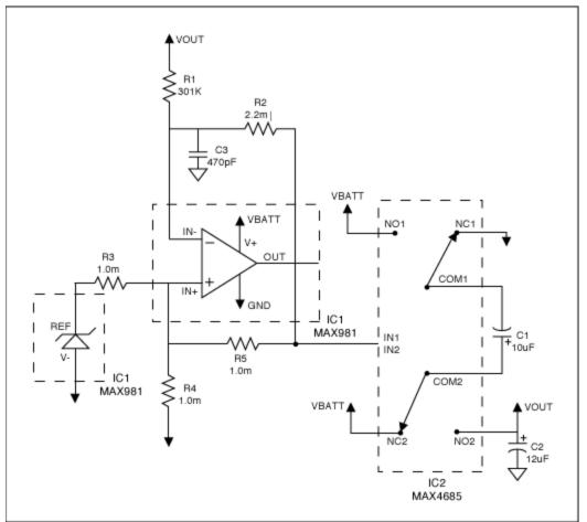
Figure 1. Low-Iq regulated charge pump.
