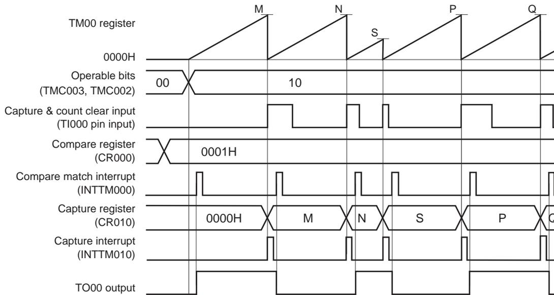
This is an application example where the TO00 output level is inverted when the count value has been captured & cleared.
