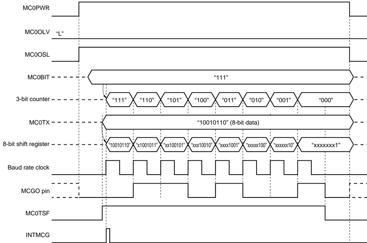
Figure 16-9. Timing of Bit Sequential Buffer Mode (LSB First) (3/4)
