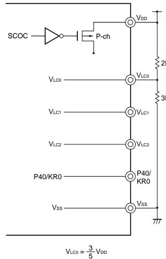
**Note** Connect  $V_{LC1}$  and  $V_{LC2}$  directly to GND or  $V_{LC0}$ .
