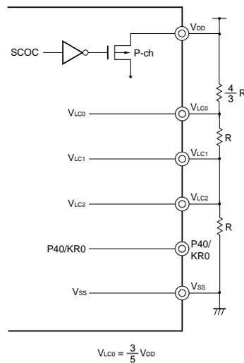
Figure 15-24. Examples of LCD Drive Power Connections (External Resistance Division Method) (2/2)
