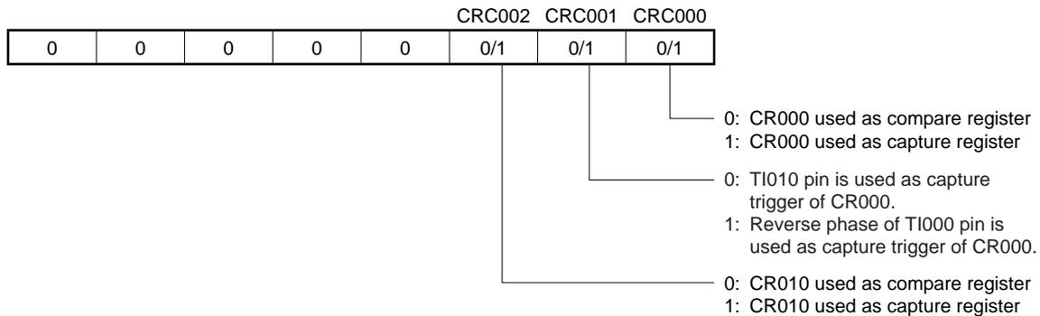
(c) 16-bit timer output control register 00 (TOC00)
