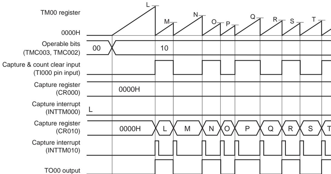
This is an application example where the count value is captured to CR010, TM00 is cleared, and the TO00 output is inverted when the rising or falling edge of the TI000 pin is detected.
