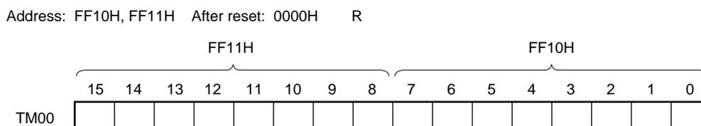
The count value of TM00 can be read by reading TM00 when the value of bits 3 and 2 (TMC003 and TMC002) of 16-bit timer mode control register 00 (TMC00) is other than 00. The value of TM00 is 0000H if it is read when TMC003 and TMC002 = 00.
