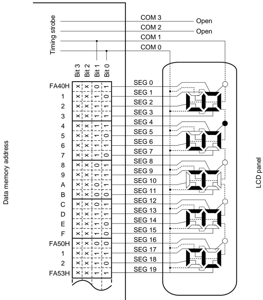
x: Can always be used to store any data because the two-time-slice mode is being used.
