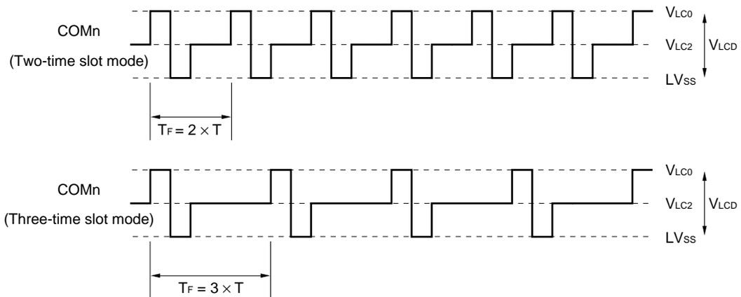
T: One LCD clock period      T<sub>F</sub>: Frame frequency
