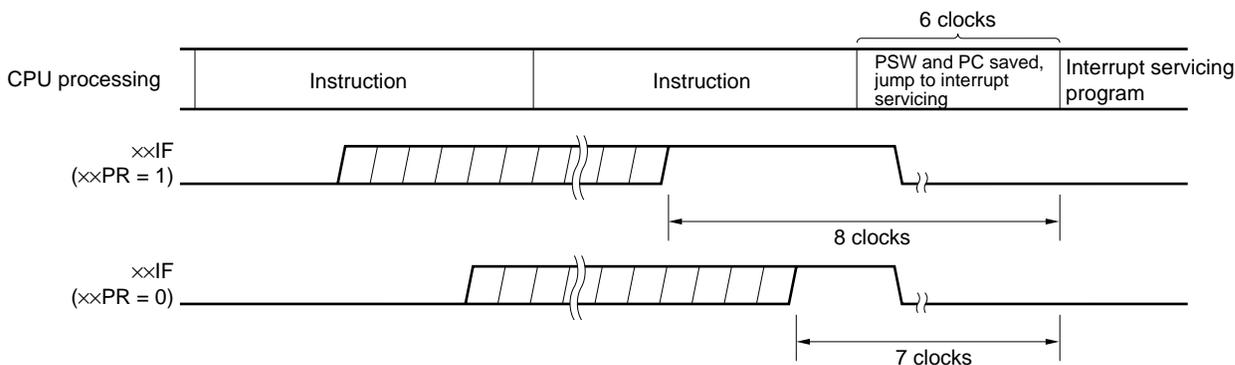
Remark 1 clock:  $1/f_{\text{CPU}}$  ( $f_{\text{CPU}}$ : CPU clock)
