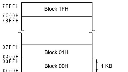
Correspondence between the address values and block numbers in the flash memory are shown below.
