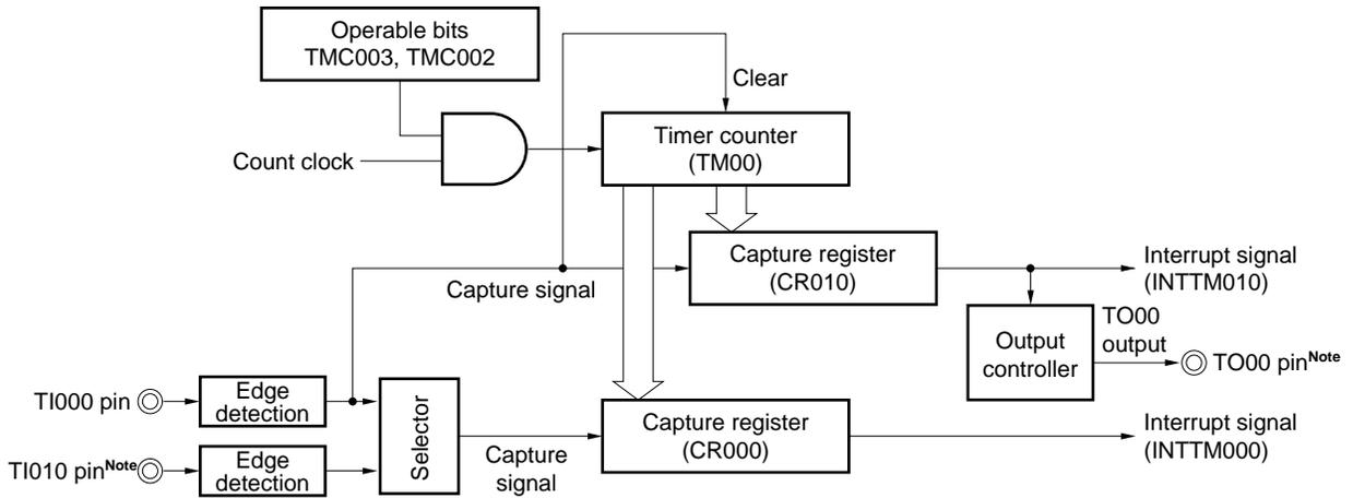
**Note** The timer output (TO00) cannot be used when detecting the valid edge of the TI010 pin is used.
