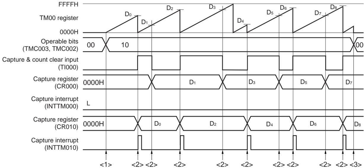
Figure 6-53. Example of Software Processing for Pulse Width Measurement (2/2)
