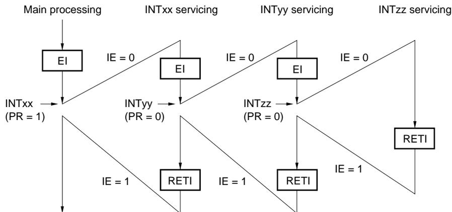
During servicing of interrupt INTxx, two interrupt requests, INTyy and INTzz, are acknowledged, and multiple interrupt servicing takes place. Before each interrupt request is acknowledged, the EI instruction must always be issued to enable interrupt request acknowledgment.
