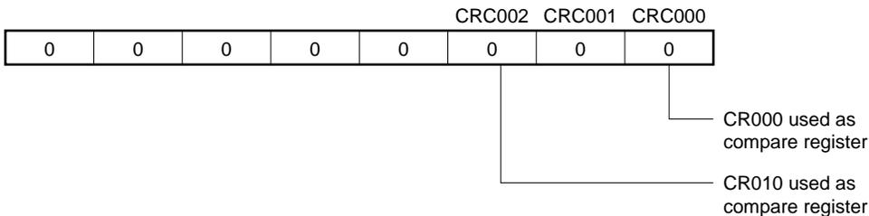
(c) 16-bit timer output control register 00 (TOC00)
