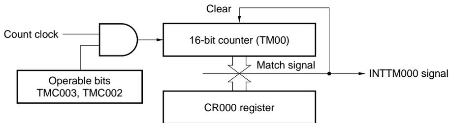
**Figure 6-13. Basic Timing Example of Interval Timer Operation**
