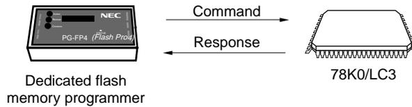
The flash memory control commands of the 78K0/LC3 are listed in the table below. All these commands are issued from the programmer and the 78K0/LC3 perform processing corresponding to the respective commands.
