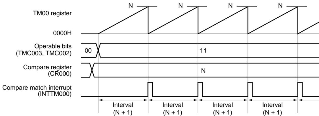
Figure 6-14. Example of Register Settings for Interval Timer Operation
