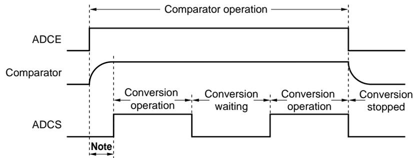
**Note** To stabilize the internal circuit, the time from the rising of the ADCE bit to the falling of the ADCS bit must be 1  $\mu$ s or longer.
