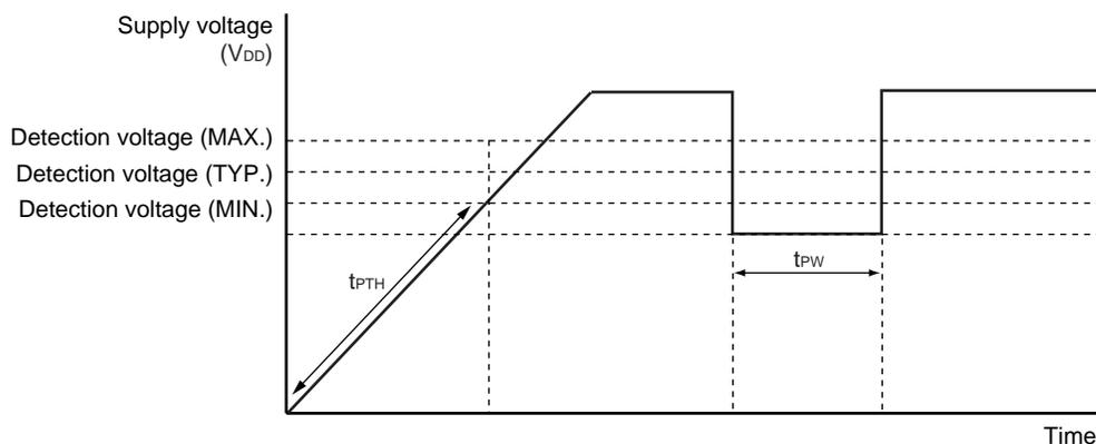
Supply Voltage Rise Time ( $T_A = -40$  to  $+85^\circ\text{C}$ ,  $V_{SS} = 0$  V)
