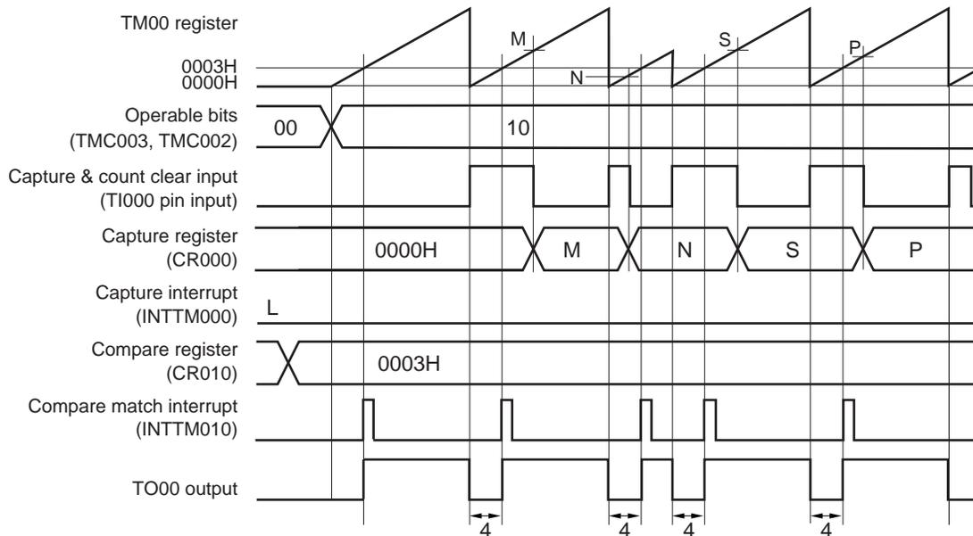
This is an application example where the width set to CR010 (4 clocks in this example) is to be output from the TO00 pin when the count value has been captured & cleared.
