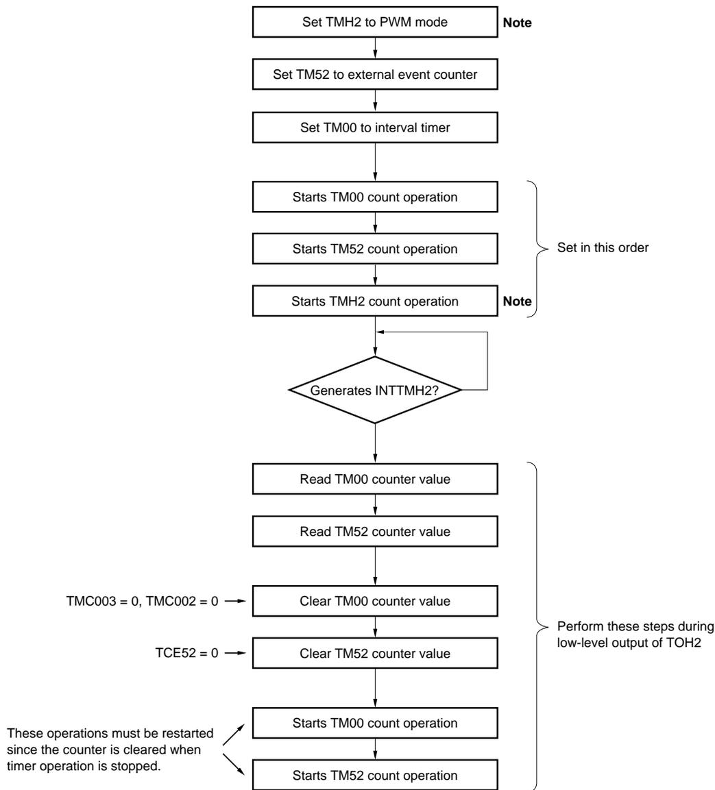
**Note** This setting is not required if input enable for the TI52 pin is not controlled.
