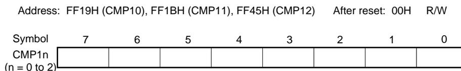
**Caution** In the PWM output mode and carrier generator mode, be sure to set CMP1n when starting the timer count operation (TMHEn = 1) after the timer count operation was stopped (TMHEn = 0) (be sure to set again even if setting the same value to CMP1n).
