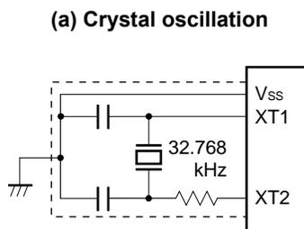
**Caution** 1. When using the X1 oscillator and XT1 oscillator, wire as follows in the area enclosed by the broken lines in the Figures 5-10 and 5-11 to avoid an adverse effect from wiring capacitance.
