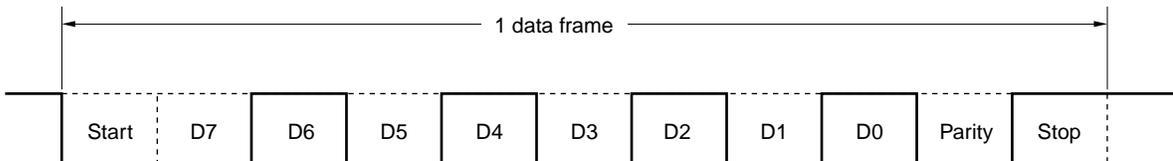
3. Data length: 8 bits, MSB first, Parity: Even parity, Stop bit: 1 bit, Communication data: 55H, Tx/D6 pin inverted output
