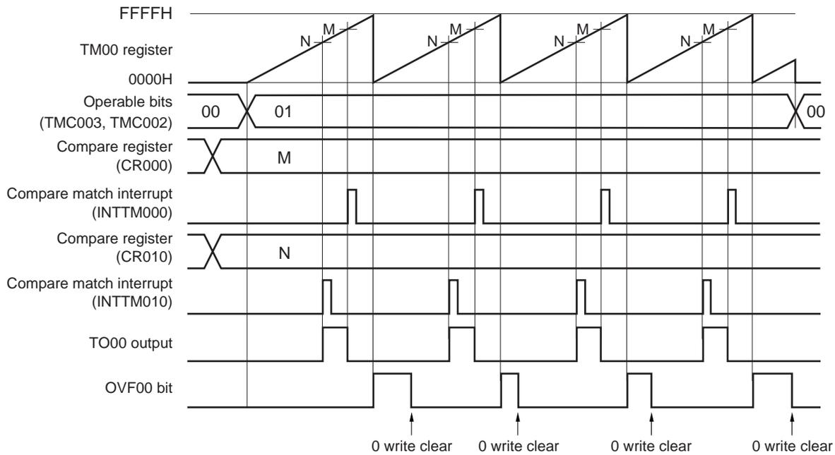
This is an application example where two compare registers are used in the free-running timer mode. The TO00 output level is reversed each time the count value of TM00 matches the set value of CR000 or CR010. When the count value matches the register value, the INTTM000 or INTTM010 signal is generated.
