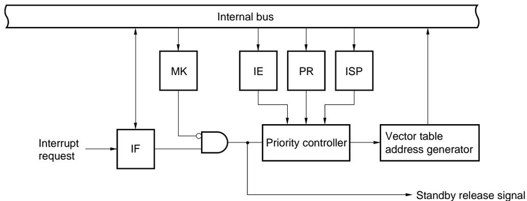
(B) External maskable interrupt (INTP0 to INTP3)
