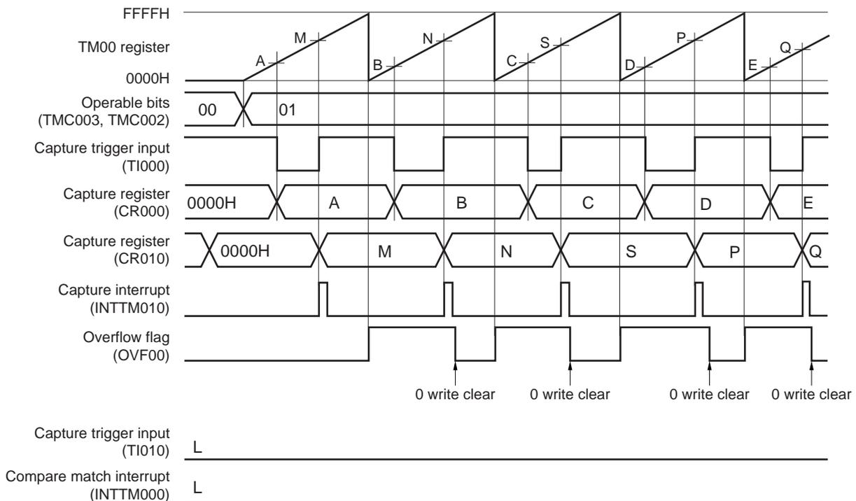
**(3) Measuring the pulse width by using one input signal of the TI000 pin (clear & start mode entered by the TI000 pin valid edge input)**
