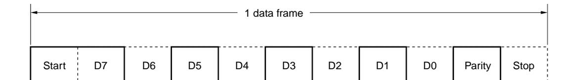
4. Data length: 7 bits, LSB first, Parity: Odd parity, Stop bit: 2 bits, Communication data: 36H
