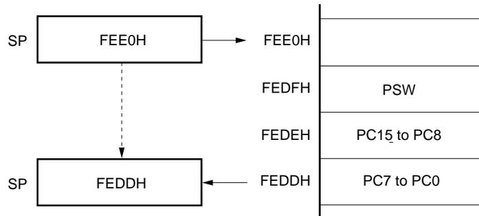
Figure 3-13. Data to Be Restored from Stack Memory
