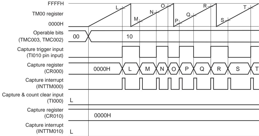
This is a timing example where an edge is not input to the TI000 pin, in an application where the count value is captured to CR000 when the rising or falling edge of the TI010 pin is detected.
