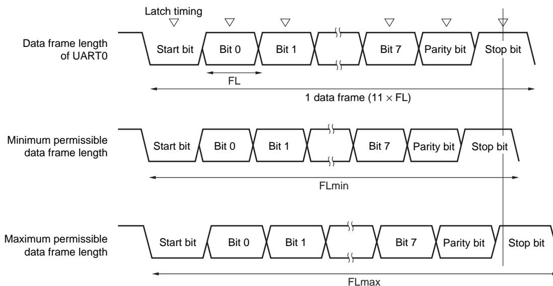
As shown in Figure 13-13, the latch timing of the receive data is determined by the counter set by baud rate generator control register 0 (BRGC0) after the start bit has been detected. If the last data (stop bit) meets this latch timing, the data can be correctly received.
