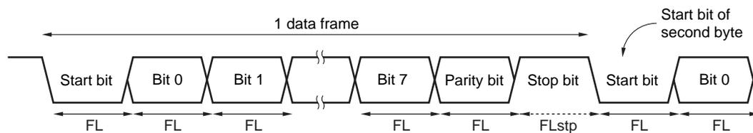
Where the 1-bit data length is  $FL$ , the stop bit length is  $FL_{stp}$ , and base clock frequency is  $f_{XCLK6}$ , the following expression is satisfied.
