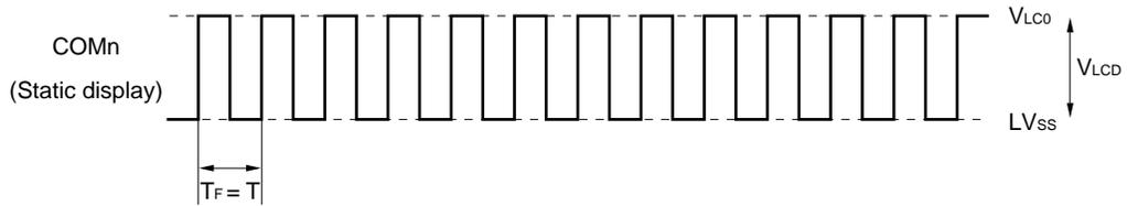
T: One LCD clock period      T<sub>F</sub>: Frame frequency
