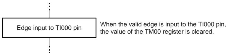
**Note** Care must be exercised when setting TOC00. For details, see 6.3 (3) 16-bit timer output control register 00 (TOC00).
