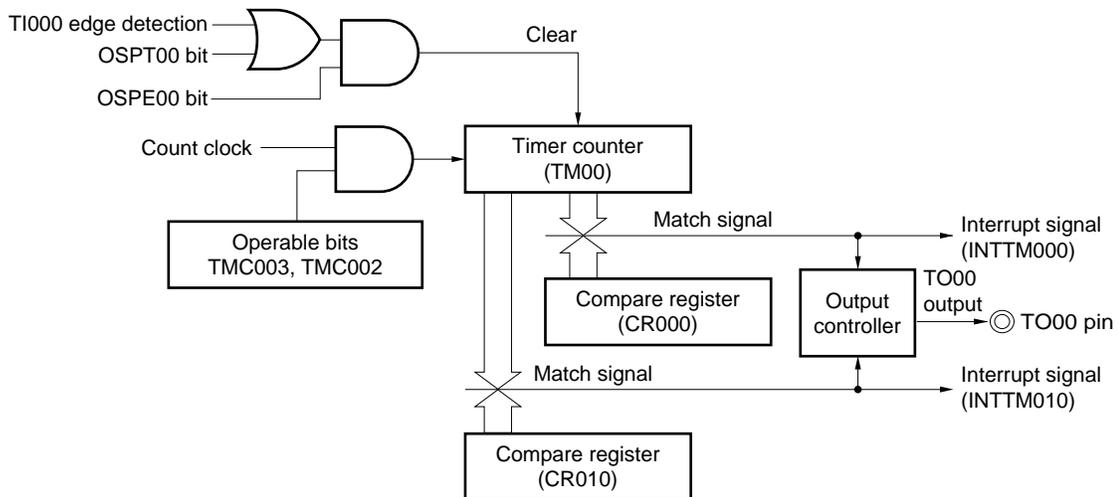
Figure 6-45. Example of Register Settings for One-Shot Pulse Output Operation (1/2)
