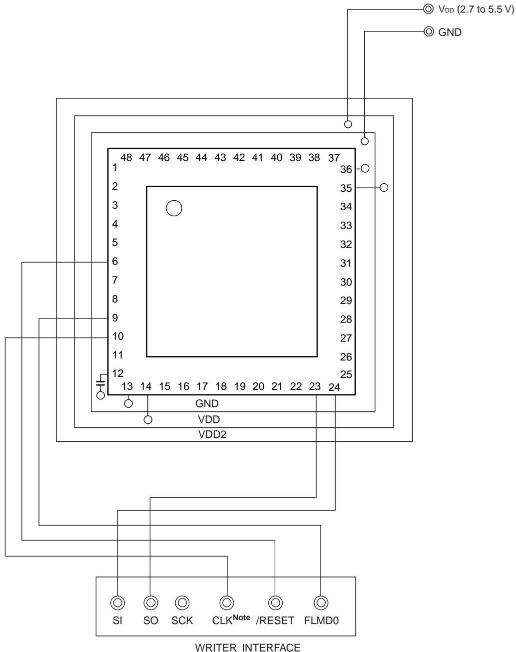
**Note** The above figure illustrates an example of wiring when using the clock output from the PG-FP4 or FL-PR4. When using the clock output from the PG-FPL3 or FP-LITE3, connect CLK to X1/P121 (pin 11), and connect its inverted signal to X2/EXCLK/P122 (pin 10).
