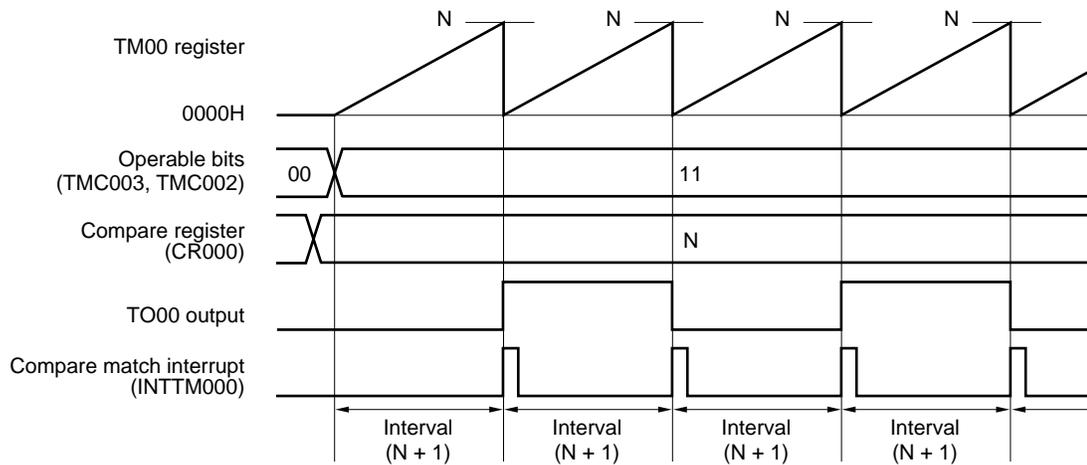
Figure 6-18. Example of Register Settings for Square Wave Output Operation
