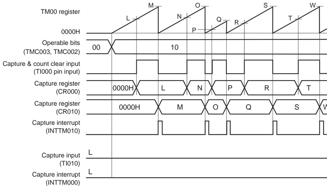
This is an application example where the pulse width of the signal input to the TI000 pin is measured.
