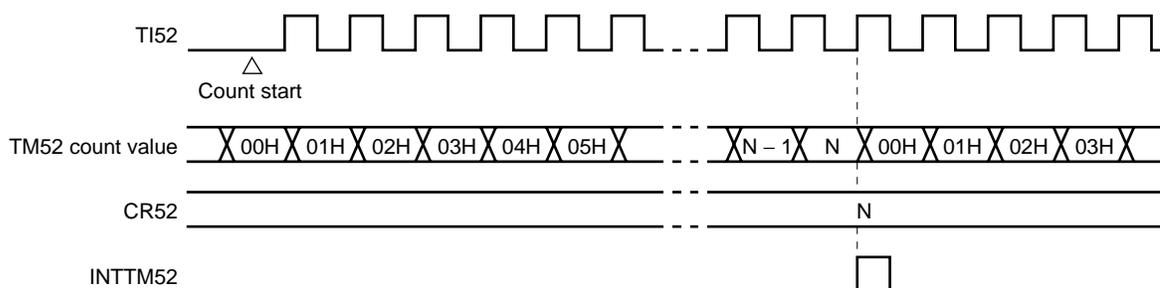
**Remark 1.** 8-bit timer/event counter 52 (TM52) can be used as a 24-bit timer/event counter, by connecting it with 16-bit timer/event counter (TM00) in cascade. Also, input enable of TM52 can be controlled via TMH2. For details, see **6.4.9 External 24-bit event counter operation**.
