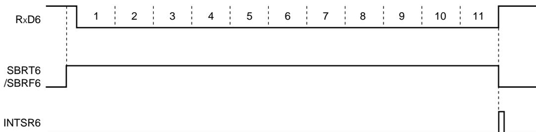
**2. SBF reception error (stop bit is detected with a width of 10.5 bits or less)**
