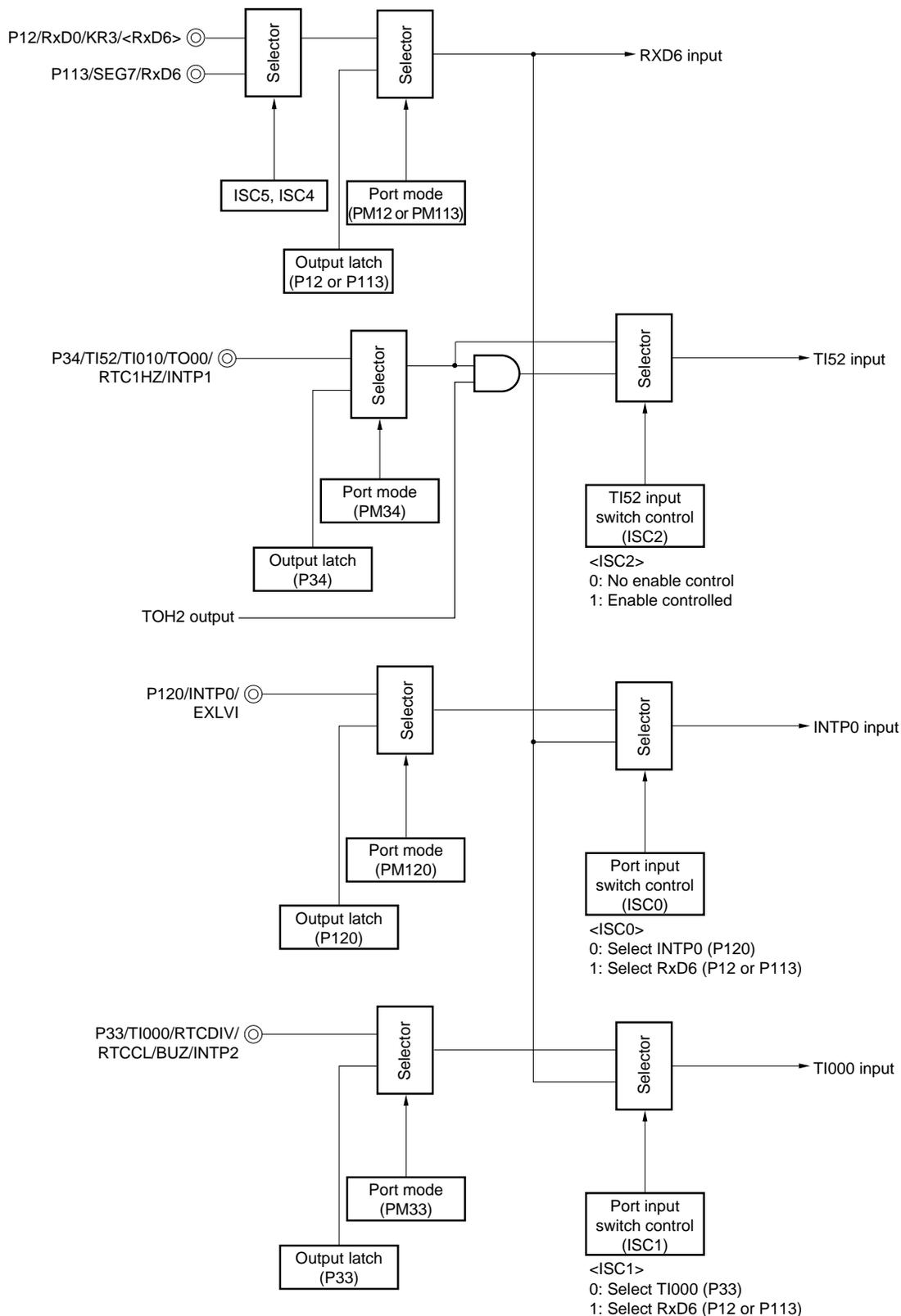
**Remark** ISC0, ISC1, ISC2, ISC4, ISC5: Bits 0, 1, 2, 4 and 5 of the input switch control register (ISC) (see **Figure 14-11**)
