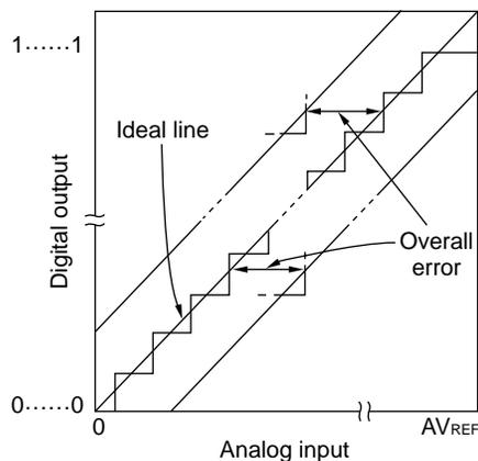
Figure 12-15. Quantization Error
