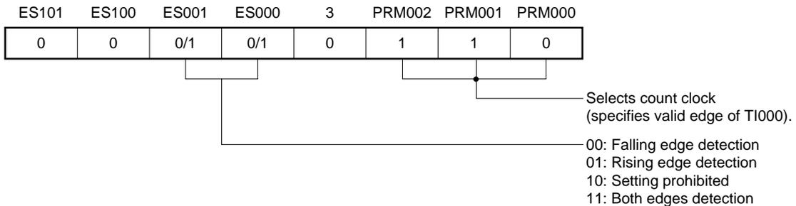
**Figure 6-21. Example of Register Settings in External Event Counter Mode (2/2)****(e) 16-bit timer counter 00 (TM00)**
