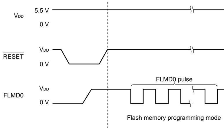
**Table 24-5. Relationship Between FLMDO Pin and Operation Mode After Reset Release**
