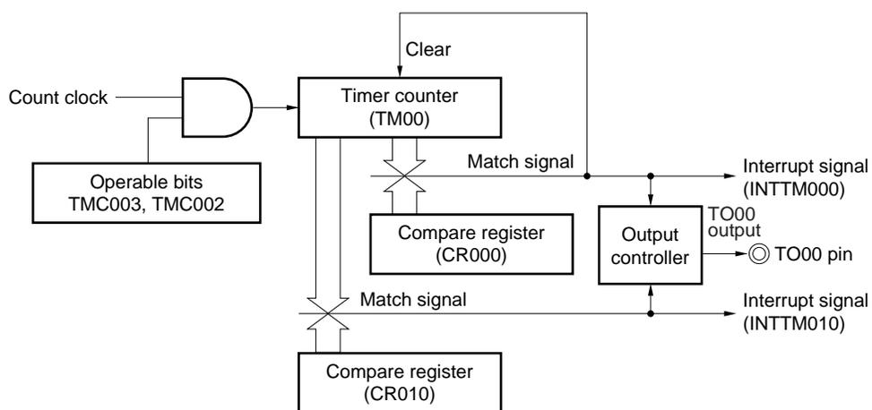
Figure 6-42. Example of Register Settings for PPG Output Operation
