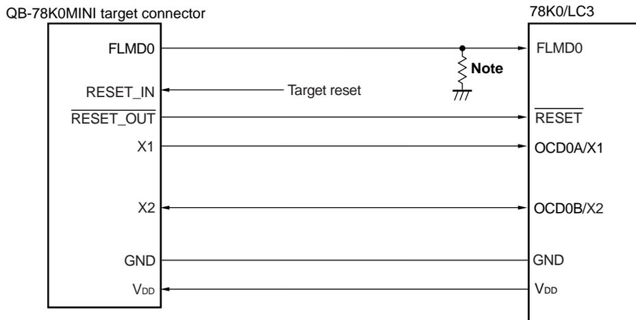
**Note** Make pull-down resistor 470 Ω or more (10 kΩ: recommended).
