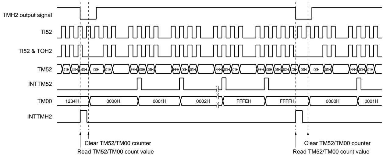
Figure 6-56. Operation Flowchart of External 24-bit Event Counter
