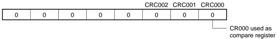
(c) 16-bit timer output control register 00 (TOC00)
