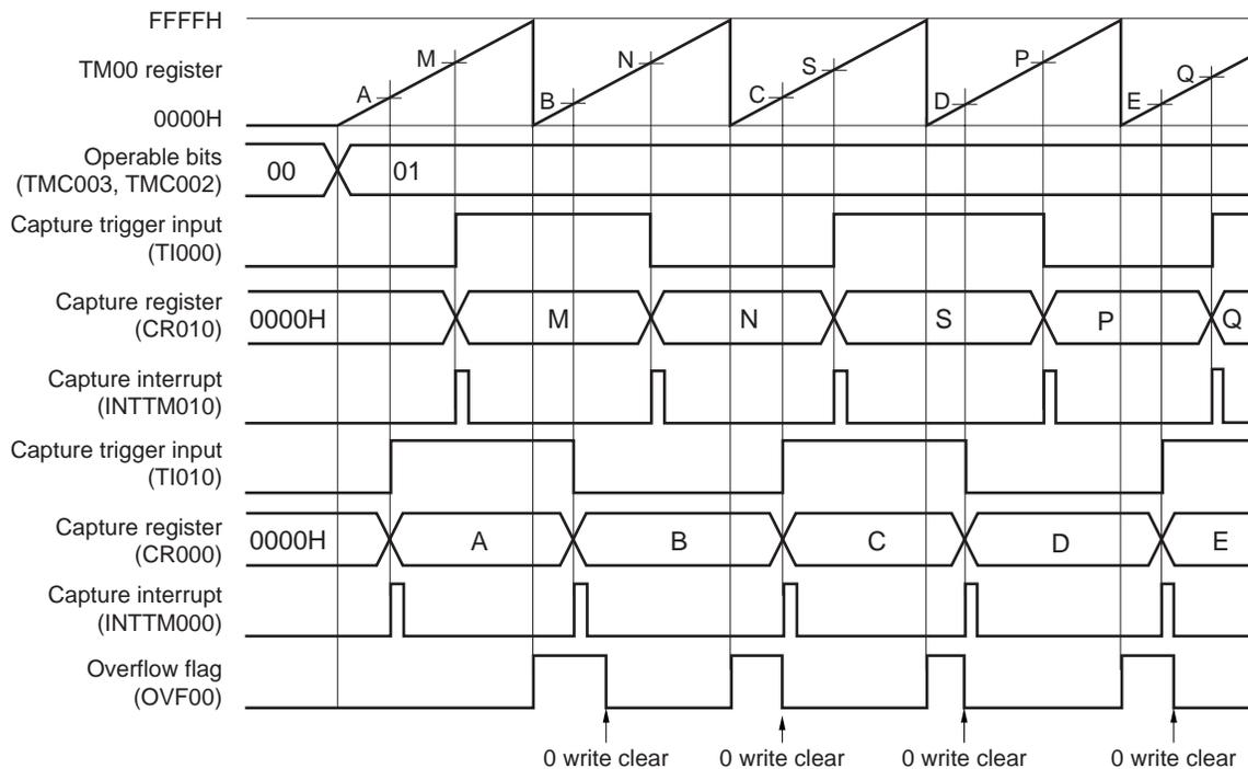
**(2) Measuring the pulse width by using one input signal of the TI000 pin (free-running mode)**
