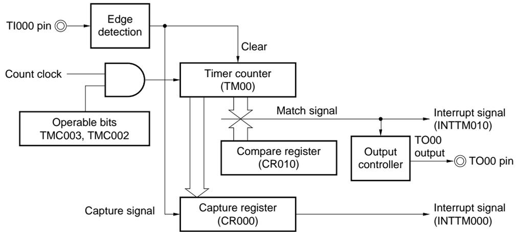
**Figure 6-28. Timing Example of Clear & Start Mode Entered by TI000 Pin Valid Edge Input (CR000: Capture Register, CR010: Compare Register) (1/2)**
