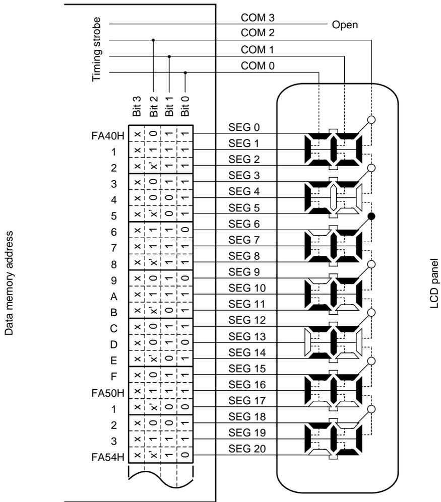
x': Can be used to store any data because there is no corresponding segment in the LCD panel.
