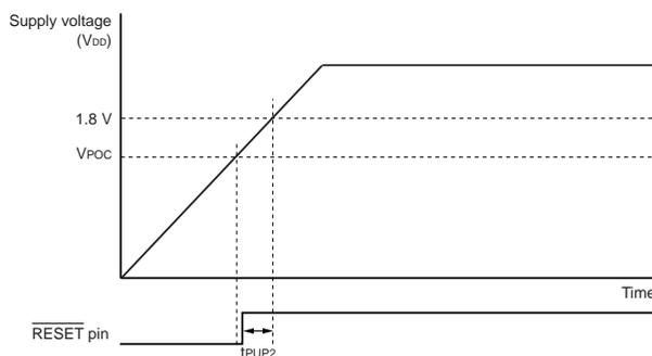
2.7 V POC Circuit Characteristics ( $T_A = -40$  to  $+85^\circ\text{C}$ ,  $V_{SS} = 0$  V)
