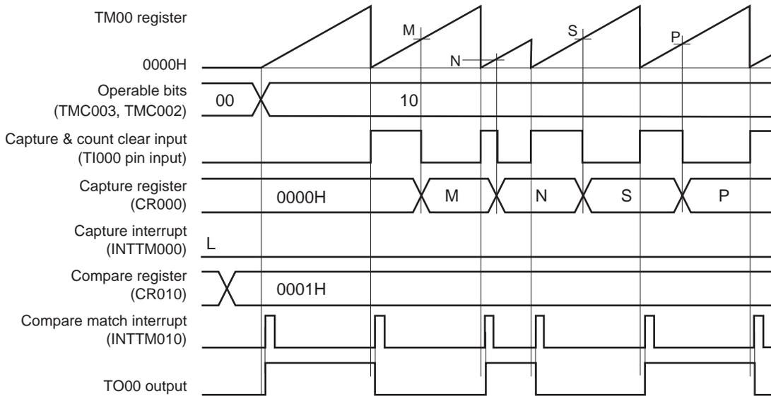
This is an application example where the TO00 output level is to be inverted when the count value has been captured & cleared.
