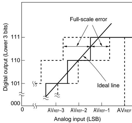
**Figure 12-18. Integral Linearity Error**
