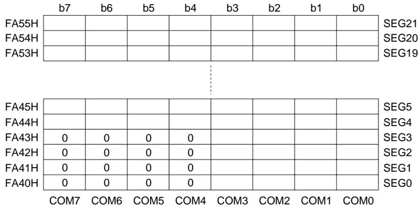
**Caution** No memory is allocated to the higher 4 bits of FA40H to FA43H. Be sure to set these bits to 0.
