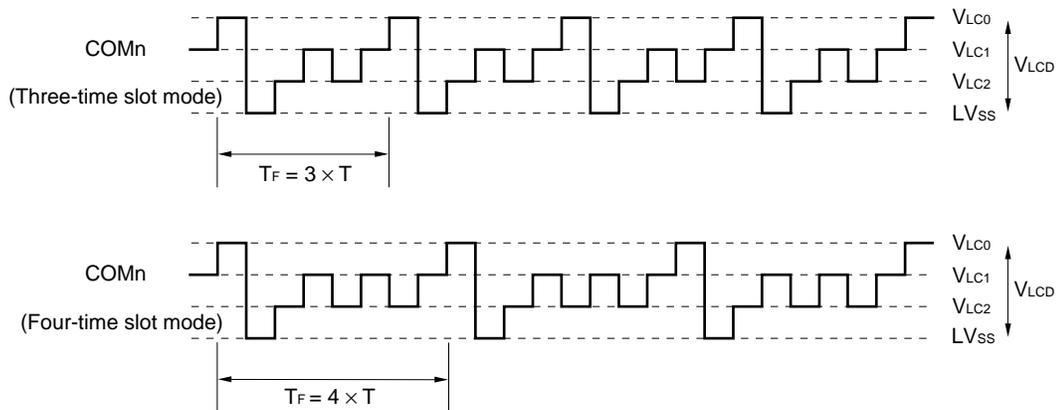
T: One LCD clock period      T<sub>F</sub>: Frame frequency
