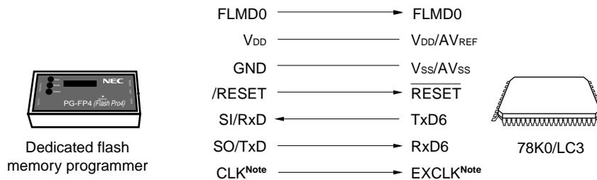
**Note** The above figure illustrates an example of wiring when using the clock output from the PG-FP4 or FL-PR4. When using the clock output from the PG-FPL3 or FP-LITE3, connect CLK to X1/P121, and connect its inverted signal to X2/EXCLK/P122.
