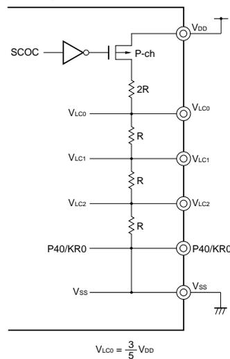
**Remark** It is recommended to use the external resistance division method when using the static display mode, in order to reduce power consumed by the voltage divider resistor.
