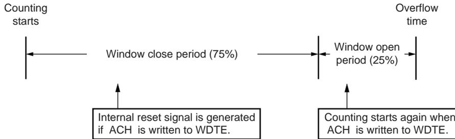
**Caution** The first writing to WDTE after a reset release clears the watchdog timer, if it is made before the overflow time regardless of the timing of the writing, and the watchdog timer starts counting again.
