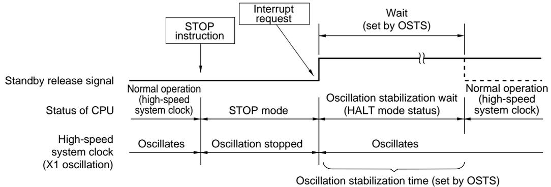
**(2) When high-speed system clock (external clock input) is used as CPU clock**
