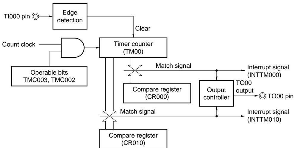
**Figure 6-24. Timing Example of Clear & Start Mode Entered by TI000 Pin Valid Edge Input (CR000: Compare Register, CR010: Compare Register)**
