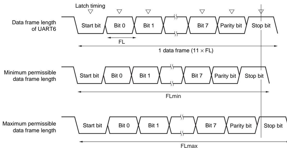
As shown in Figure 14-27, the latch timing of the receive data is determined by the counter set by baud rate generator control register 6 (BRGC6) after the start bit has been detected. If the last data (stop bit) meets this latch timing, the data can be correctly received.
