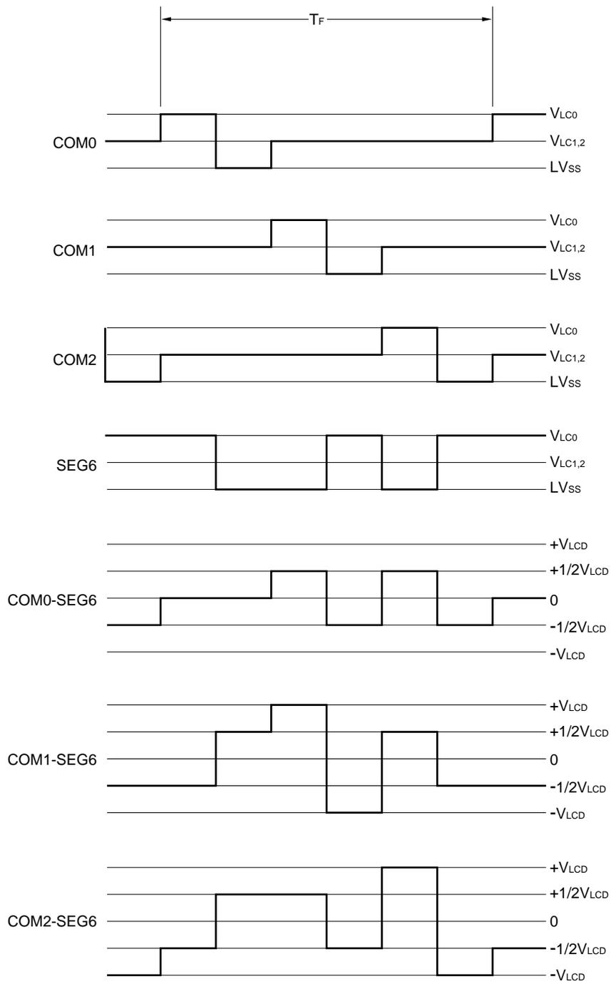
Figure 15-19. Three-Time-Slice LCD Drive Waveform Examples (1/3 Bias Method)
