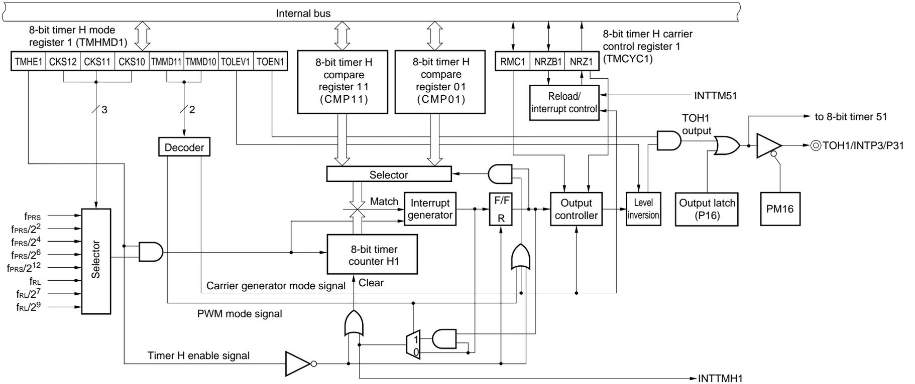
Figure 8-3. Block Diagram of 8-Bit Timer H2
