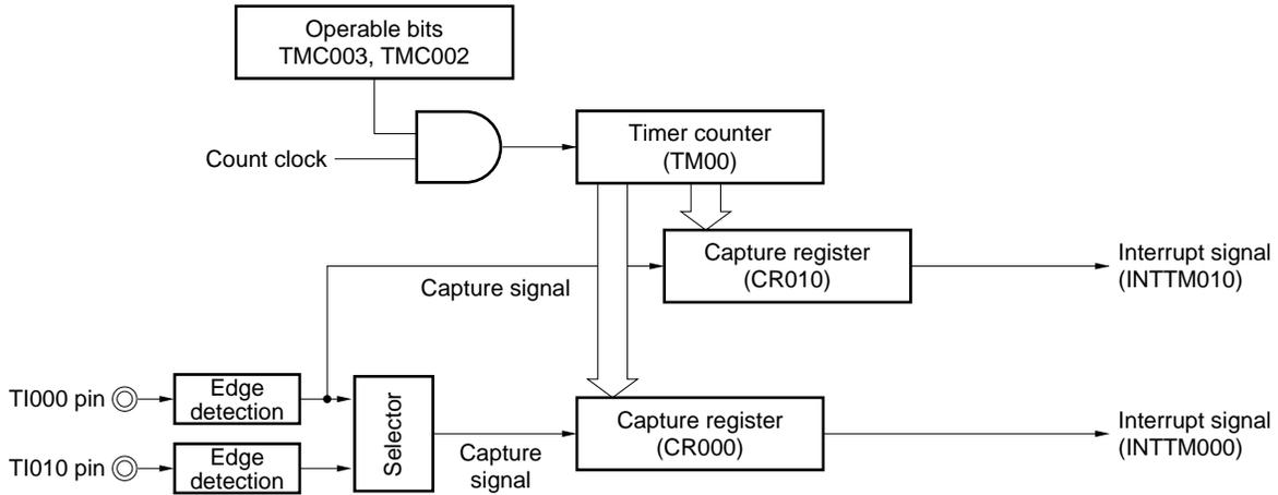
**Remark** If both CR000 and CR010 are used as capture registers in the free-running timer mode, the TO00 output level is not inverted. However, it can be inverted each time the valid edge of the TI000 pin is detected if bit 1 (TMC001) of 16-bit timer mode control register 00 (TMC00) is set to 1.
