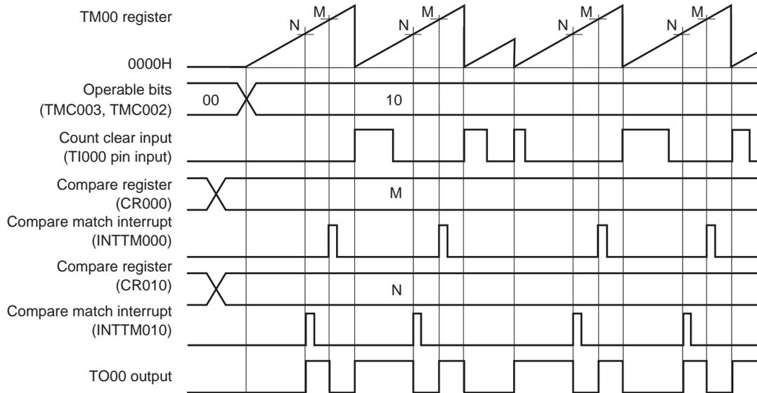
(a) and (b) differ as follows depending on the setting of bit 1 (TMC001) of the 16-bit timer mode control register 01 (TMC00).
