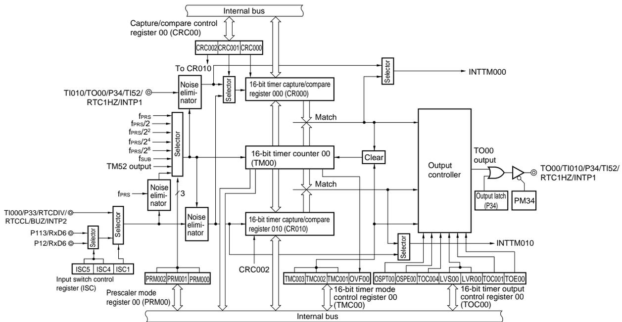
**Cautions 1.** The valid edge of TI010 and timer output (TO00) cannot be used for the P34 pin at the same time. Select either of the functions.
