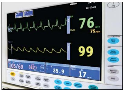
Patient monitor showing ECG and pulse oximetry readings.
