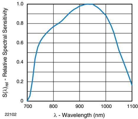
Fig. 2 - Relative Spectral Sensitivity vs. Wavelength
