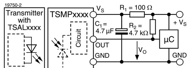
$R_1 + C_1$  recommended to suppress power supply disturbances.
