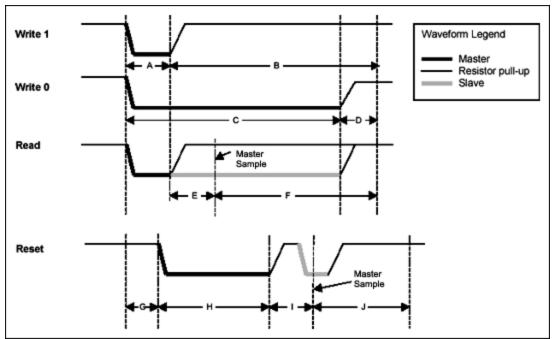
Figure 1. 1-Wire waveforms.
