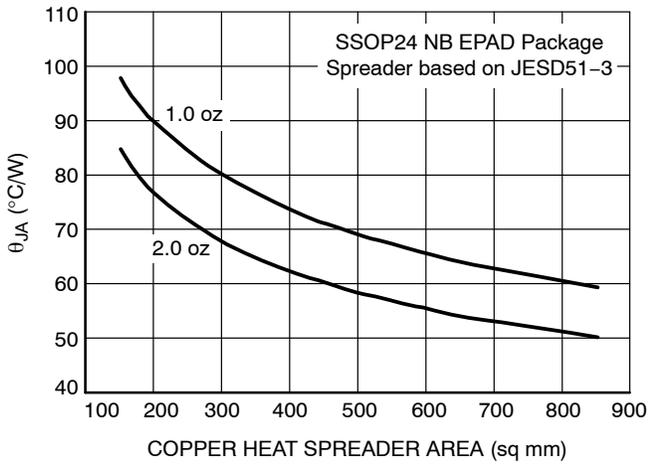
Figure 25.  $\theta_{JA}$  vs. Cu Area: SSOP24 NB EP
