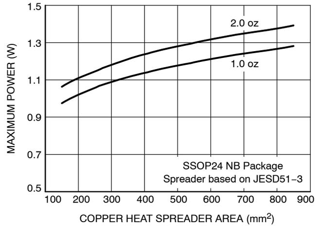
Figure 29. Power vs. Cu Area: SSOP24 NB
