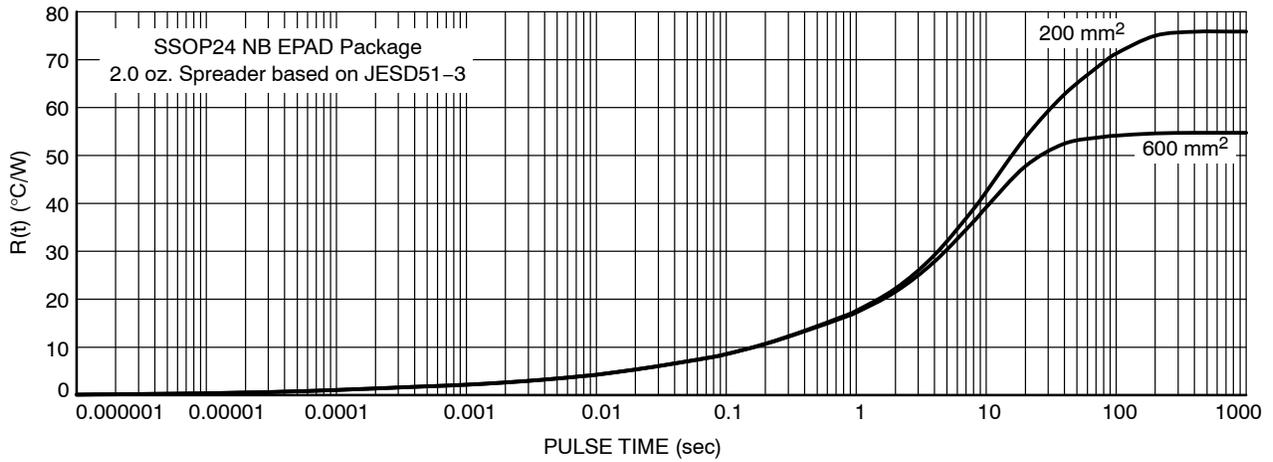
Figure 27. R(t) vs. Duty Cycle: SSOP24 NB EP
