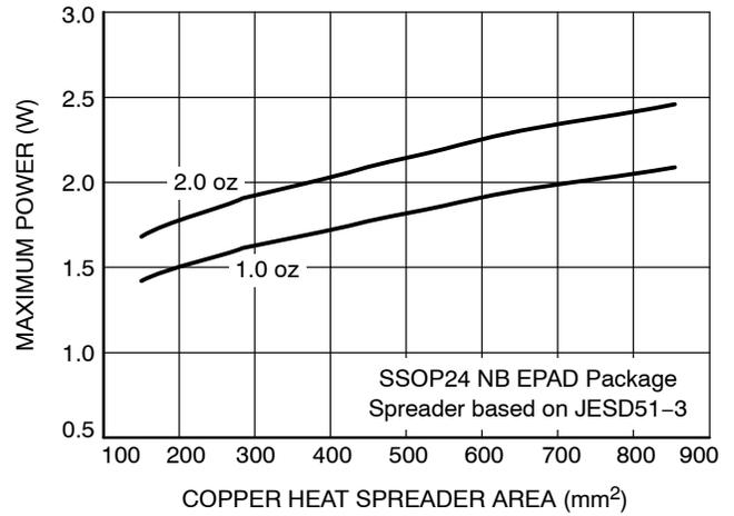
Figure 26. Power vs. Cu Area: SSOP24 NB EP
