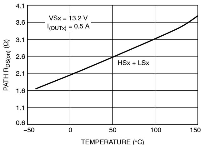
Figure 9. R<sub>DS(on)</sub> vs. Temperature
