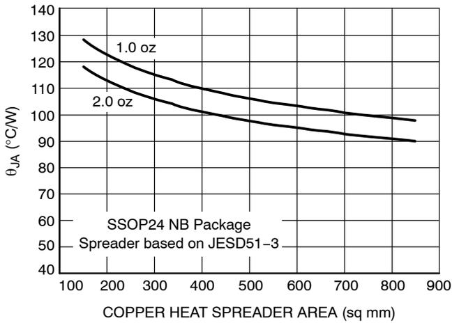
Figure 28.  $\theta_{JA}$  vs. Cu Area: SSOP24 NB
