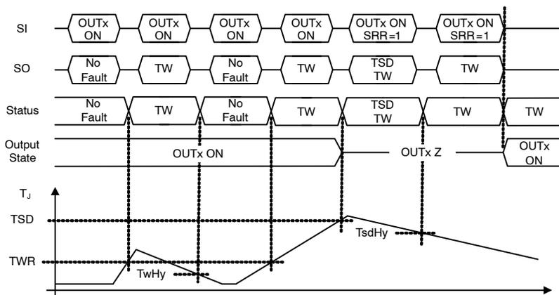
Figure 24. Thermal Warning and Shutdown Timing Diagram
