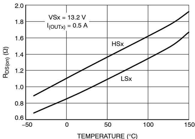
Figure 8. R<sub>DS(on)</sub> vs. Temperature
