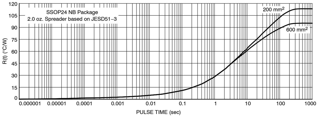
Figure 30.  $R(t)$  vs. Duty Cycle: SSOP24 NB
