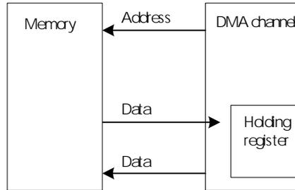
*Figure 21: DMA memory-to-memory transfer*
