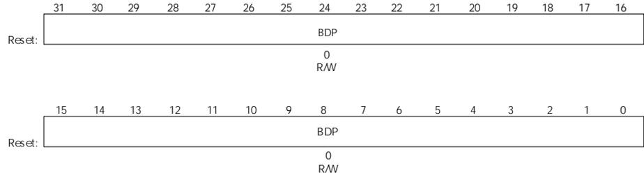
The DMA buffer descriptor pointer contains the address of the first buffer descriptor in a contiguous list of descriptors. The last descriptor in the list is identified with the W bit set in the buffer descriptor header.
