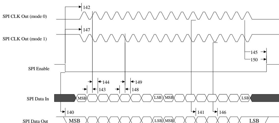
**Figure 89: SPI Slave mode 0 and 1 (two-byte transfer)**
