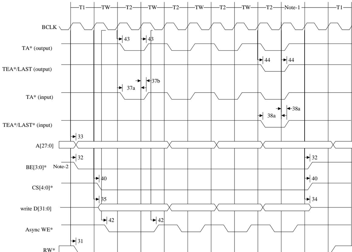
**Figure 69: SRAM Asynchronous Burst Write (WAIT = 2, BCYC = 01)**
