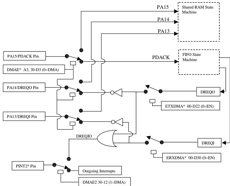
**Figure 57: ENI FIFO — Transporting data through DMA channels**
