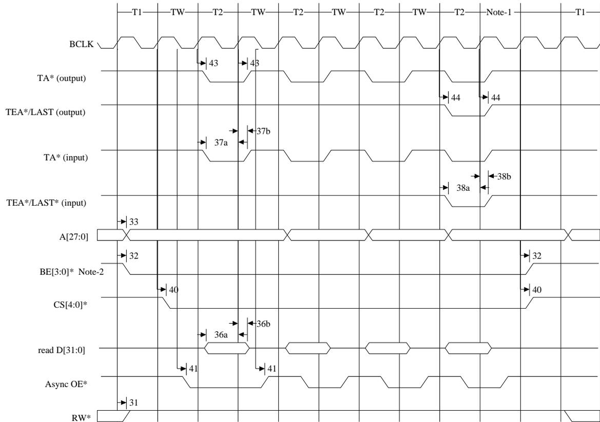
**Figure 68: SRAM Asynchronous Burst Read (WAIT = 2, BCYC = 01)**
