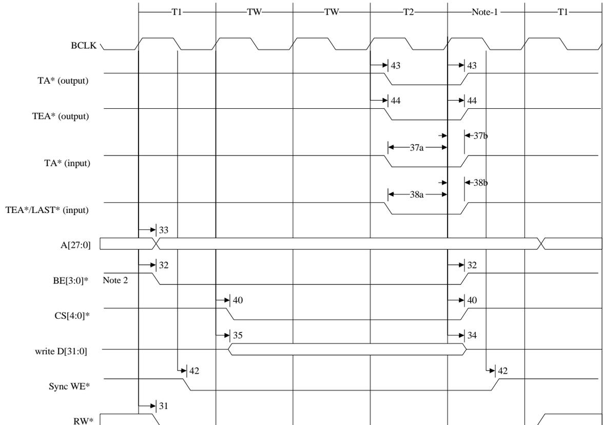
**Figure 62: SRAM Synchronous Write (WAIT = 2)**
