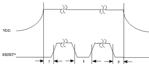
**Figure 60: RESET\* timing**
