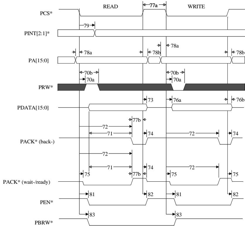
**Figure 90: ENI Shared RAM and Register Cycle timing**
