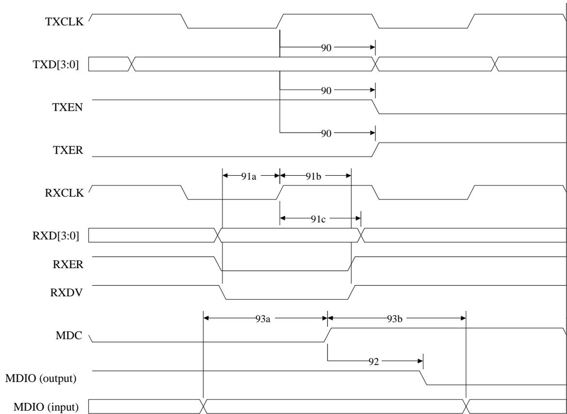
Figure 93: Ethernet timing
