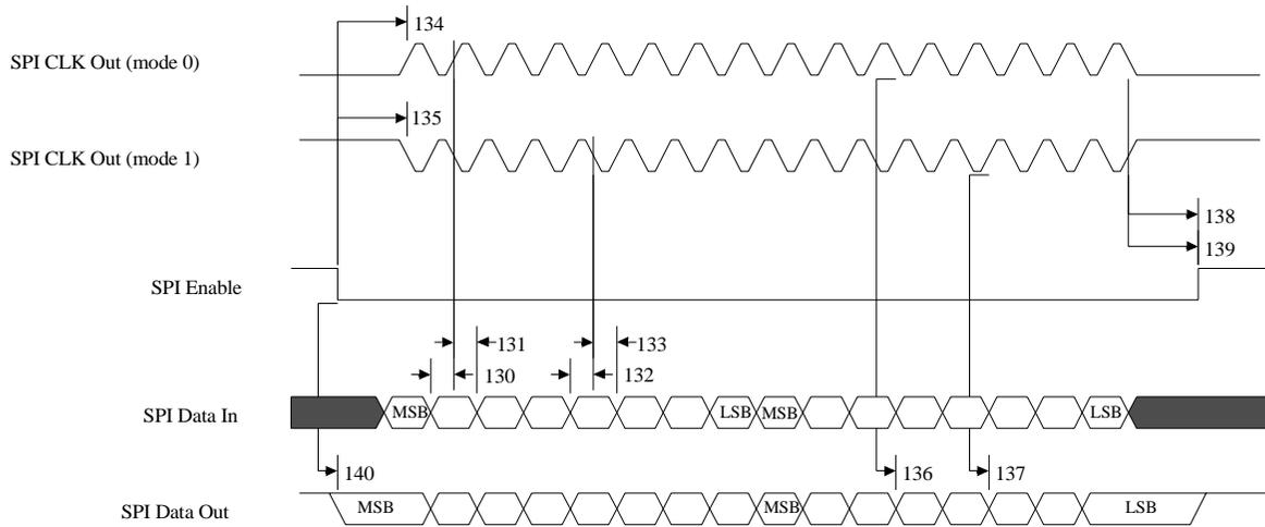
Figure 88: SPI Master mode 0 and 1 (two-byte transfer)
