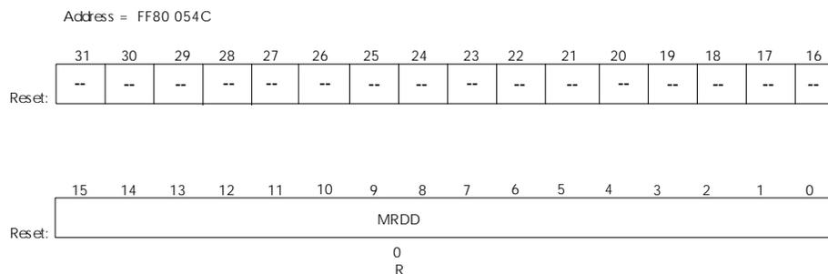
The MII Read Data register provides read data after an MII management read cycle. An MII management read cycle is executed by loading the PHY Address register, then setting the READ bit in the MII Command register to 1.
