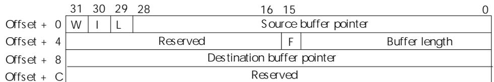
**Figure 25: DMA buffer descriptor — Memory-to-memory mode**
