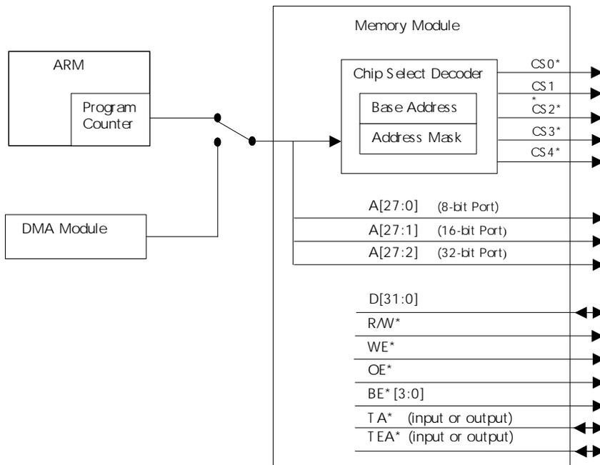
**Figure 13: SRAM chip select configuration**
