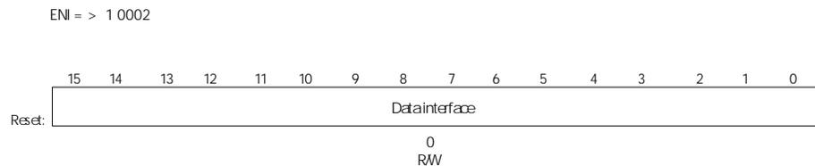
When accessing the FIFO Data register from the external ENI interface, the access timing is always the same — unlike accessing shared RAM. Because the ENI hardware does not need to arbitrate with internal resources when accessing the FIFO Data register, the access timing for this data register is fast and consistent.
