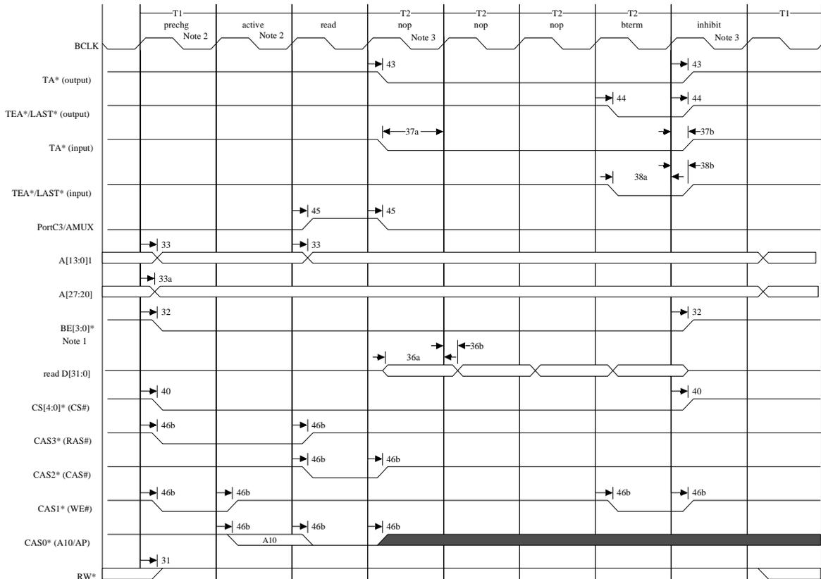
**Figure 81: SDRAM Burst Read (CAS Latency = 1)**
