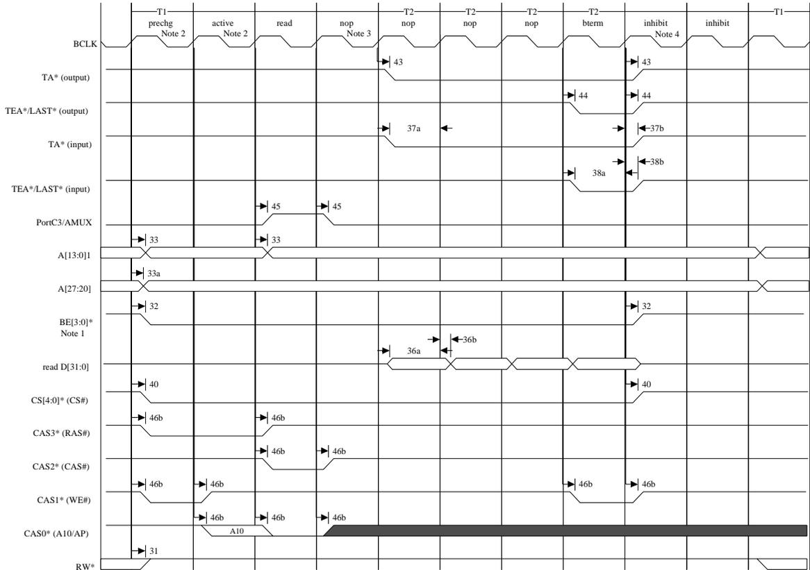
**Figure 82: SDRAM Burst Read (CAS Latency = 2)**
