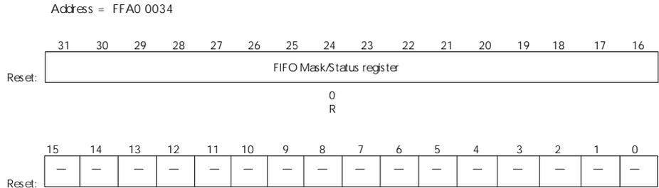
The external ENI client processor is responsible for setting the bits in the FIFO Mask/Status register (see "FIFO Mask/Status register and bit definition" on page 395). The ARM processor can read the values written by the ENI client processor by reading the ENI Pulsed Interrupt register. The lower sixteen bits in the FIFO Mask/Status register are mapped onto the upper sixteen bits of the ENI Pulsed Interrupt register.
