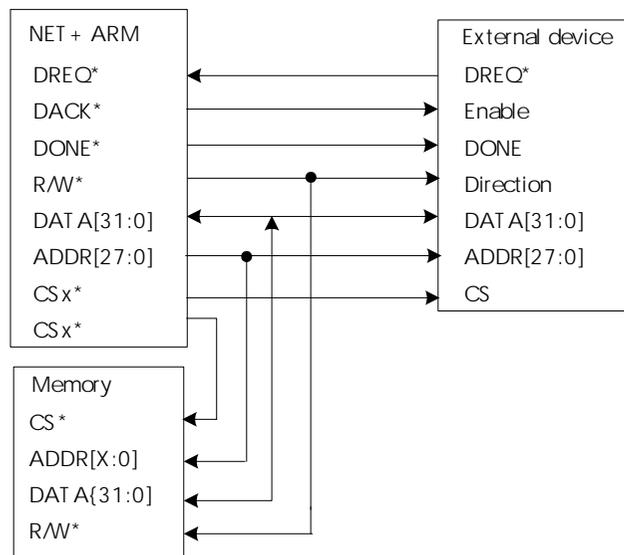
**Figure 29: Hardware needed for external memory-to-memory DMA transfers**
