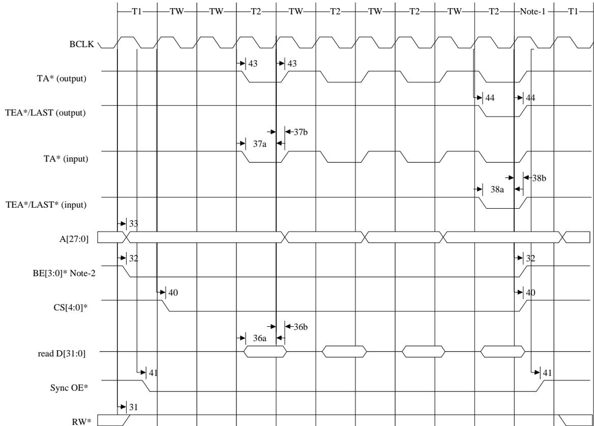
**Figure 64: SRAM Synchronous Burst Read (4-222) (WAIT = 2, BCYC = 01)**
