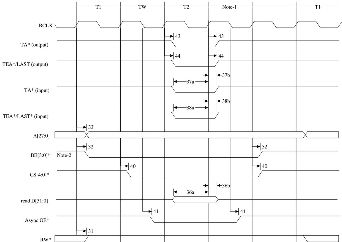
**Figure 66: SRAM Asynchronous Read (WAIT = 2)**
