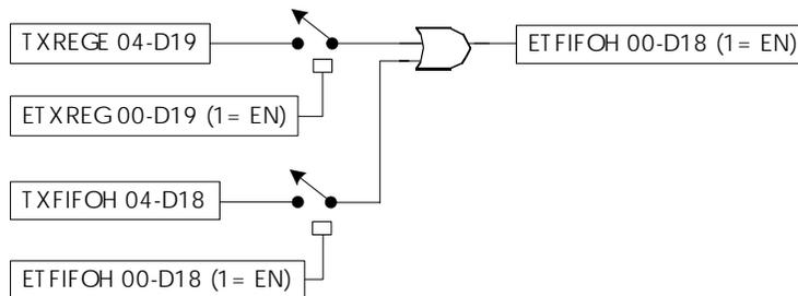
**Figure 59:** *ENI transmit FIFO interrupt process*
