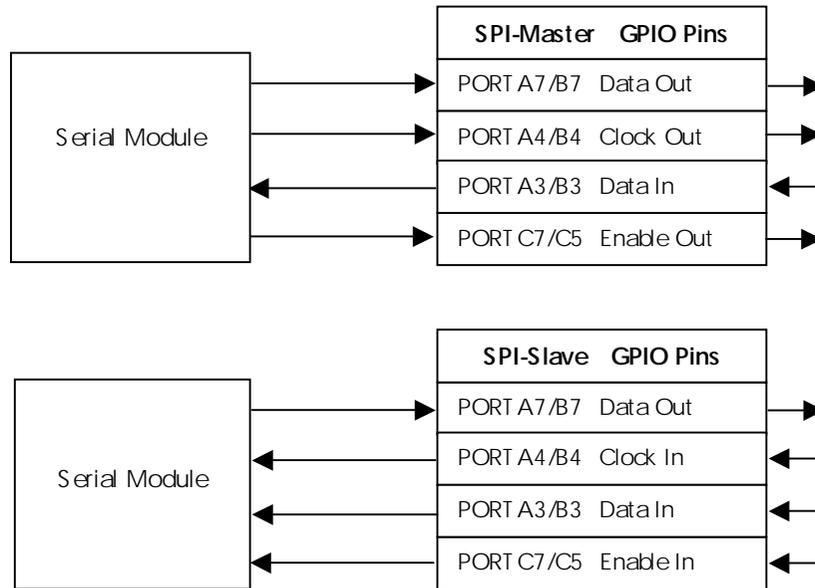
*Figure 32: SPI mode/GPIO signal relationships*
