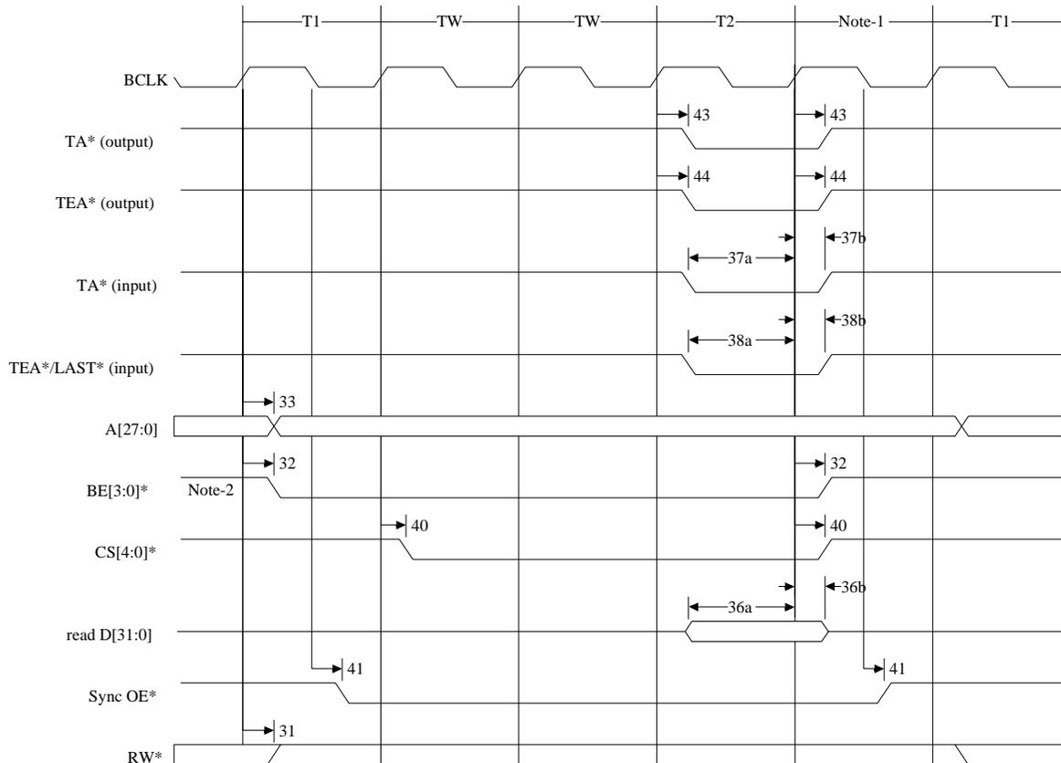
**Figure 61: SRAM Synchronous Read (WAIT = 2)**
