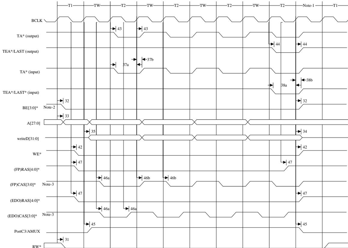
**Figure 73: Fast Page and EDO DRAM Burst Write**
