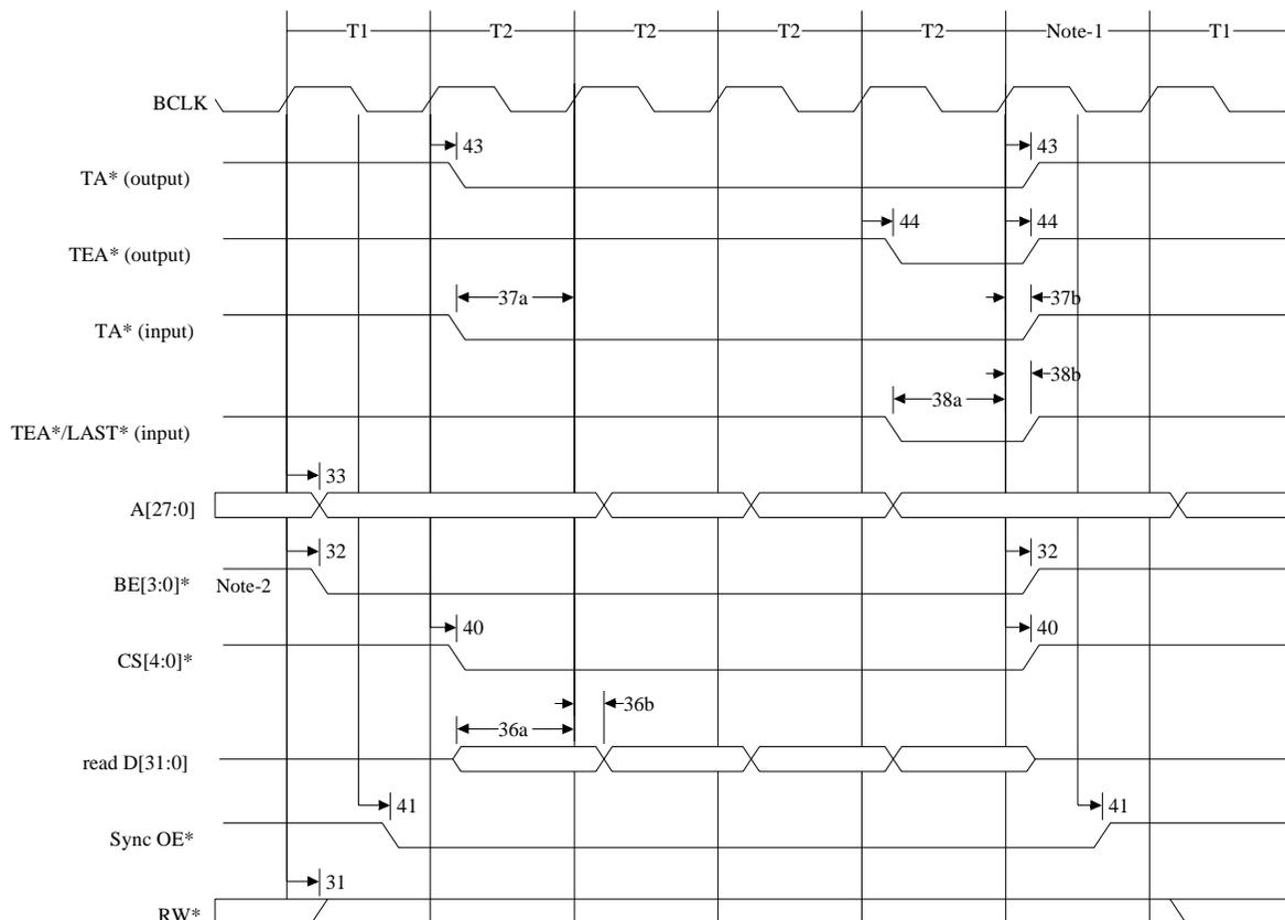
**Figure 63: SRAM Synchronous Burst Read (2-111) (WAIT = 0, BCYC = 00)**
