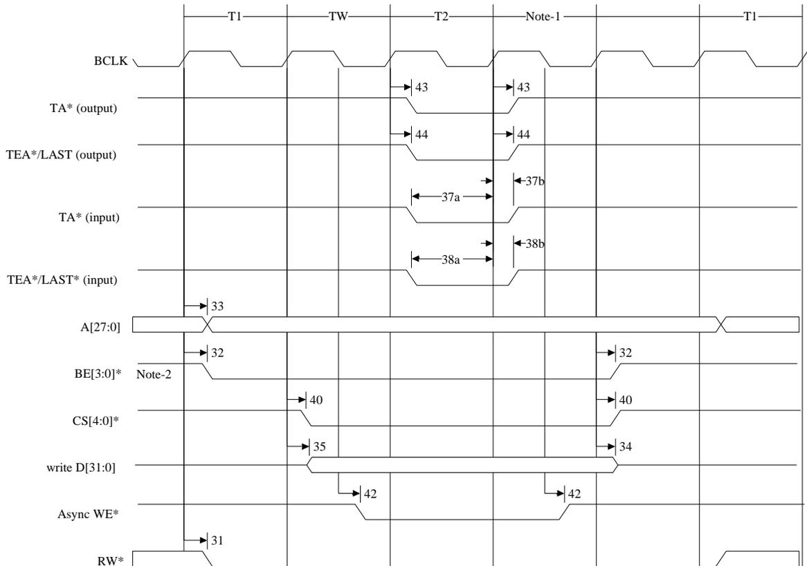
**Figure 67: SRAM Asynchronous Write (WAIT = 2)**
