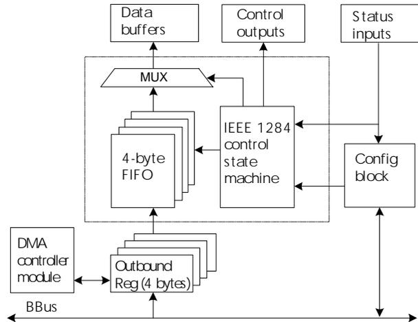
**Figure 41: IEEE 1284 host controller block diagram**
