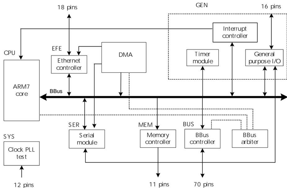
**Figure 2:** NET+20M device modules
