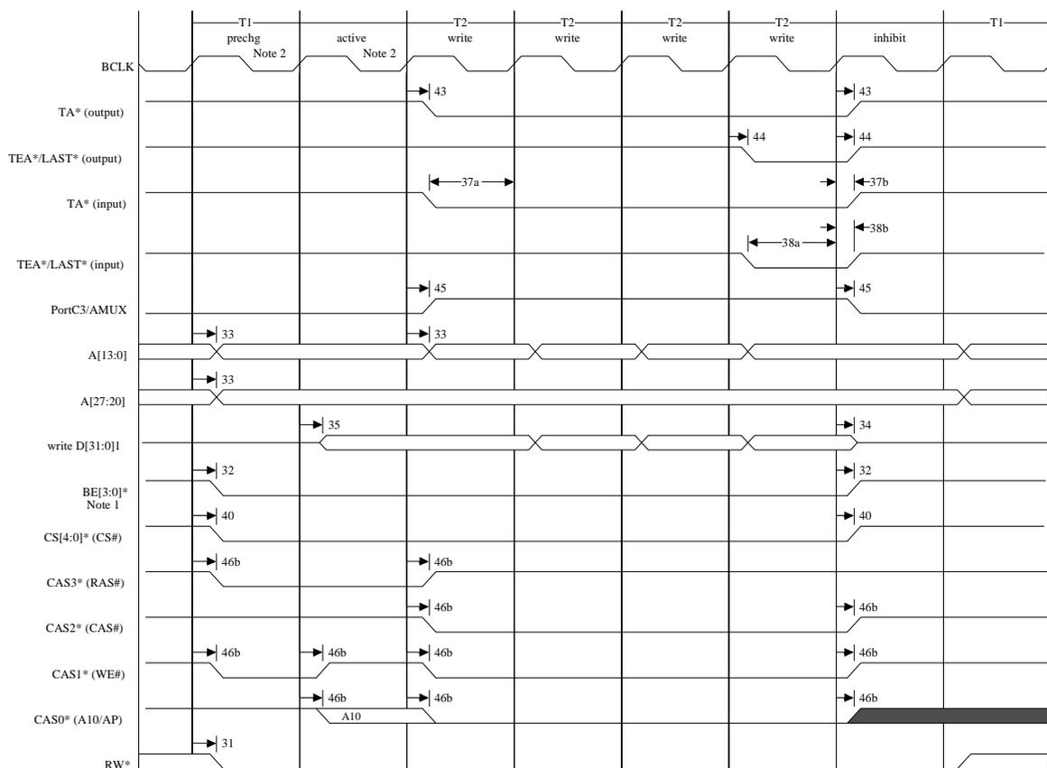
**Figure 83: SDRAM Burst Write (CAS Latency = 2)**
