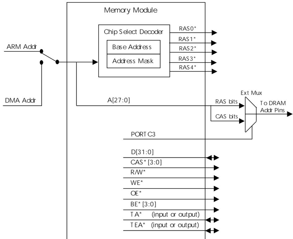
**Figure 14: External DRAM multiplexer chip select configuration**
