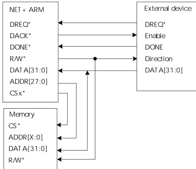
**Figure 28: Hardware needed for external fly-by DMA transfers**
