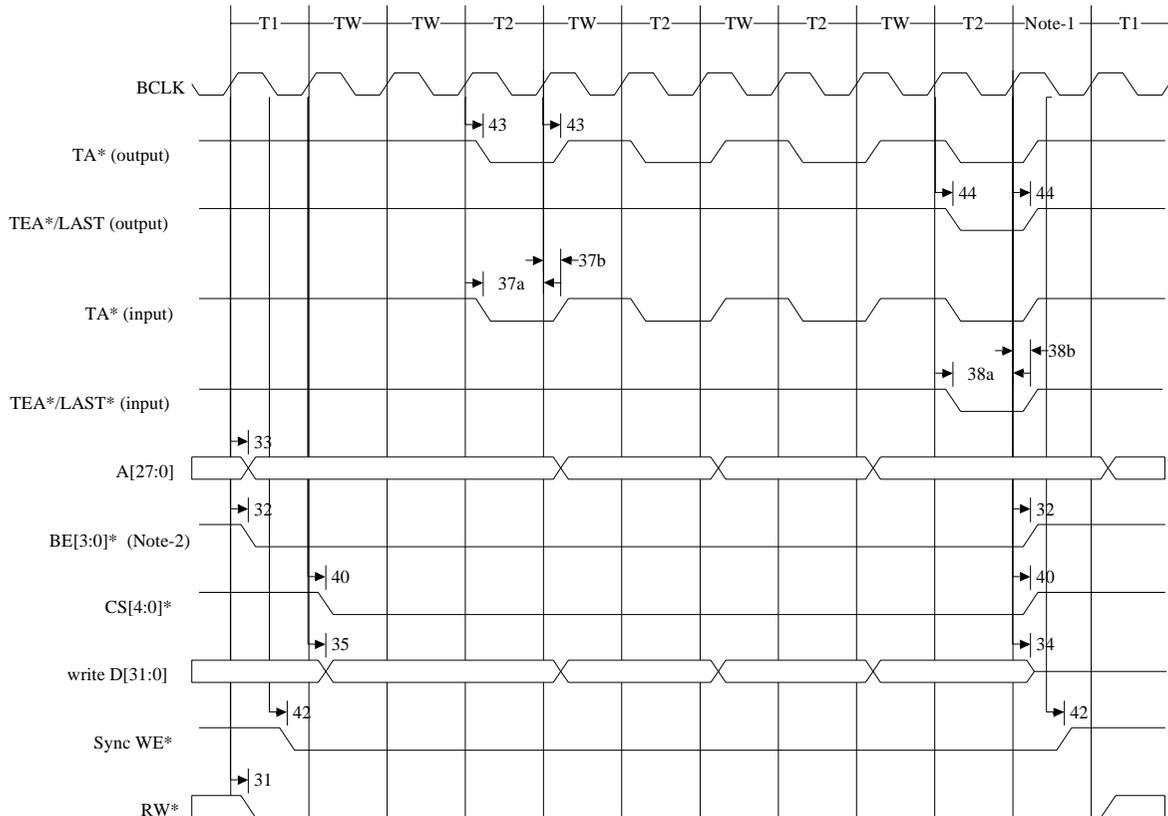
**Figure 65: SRAM Synchronous Burst Write (4-222) (WAIT = 2, BCYC = 01)**
