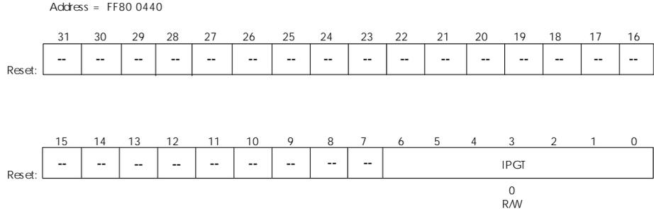
The *IPGT* (006:00), or back-to-back transmit IPG, spaces back-to-back transmit packets. The Ethernet transmit state machine has an intrinsic delay of four Ethernet clocks between packets. With the IPGT field set to 0, the IPG will be a minimum of four Ethernet clocks, or 0.16  $\mu$ S, when operating at 100BT.
