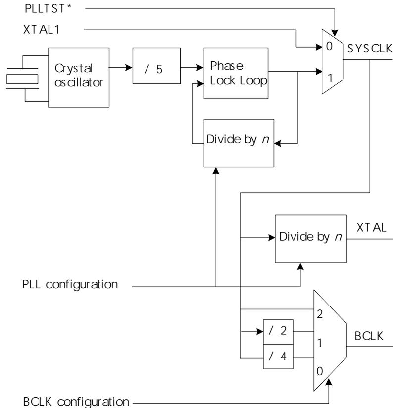
*Figure 8: NET+50 chip clock generation*
