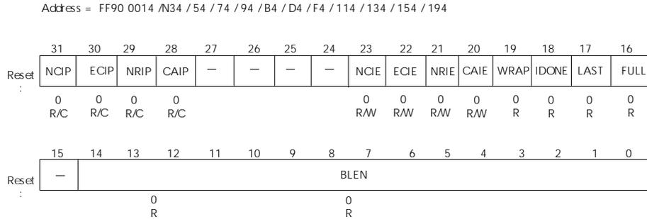
The interrupt enable (IE) bits can be set to cause an interrupt to occur when the corresponding interrupt status bit is set in the DMA Status register. The interrupt pending (IP) bits are set to indicate begin active. These bits are cleared by writing a 1 to the same bit locations.
