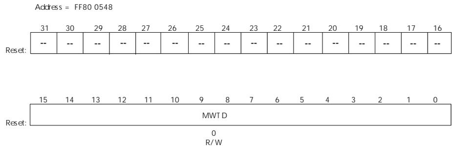
When this register is written, an MII management write cycle is performed using the 16-bit data defined in the PHY Address register by the pre-configured PHY device and PHY register addresses. The write operation is completed when the BUSY bit in the MII Indicators register returns to 0.
