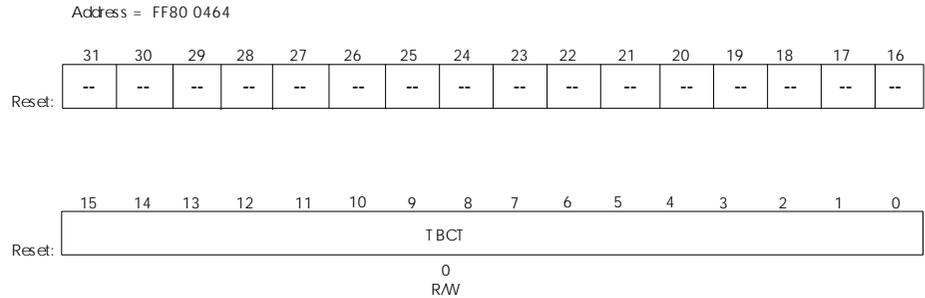
**Retransmit Byte Counter register (RETX)**
