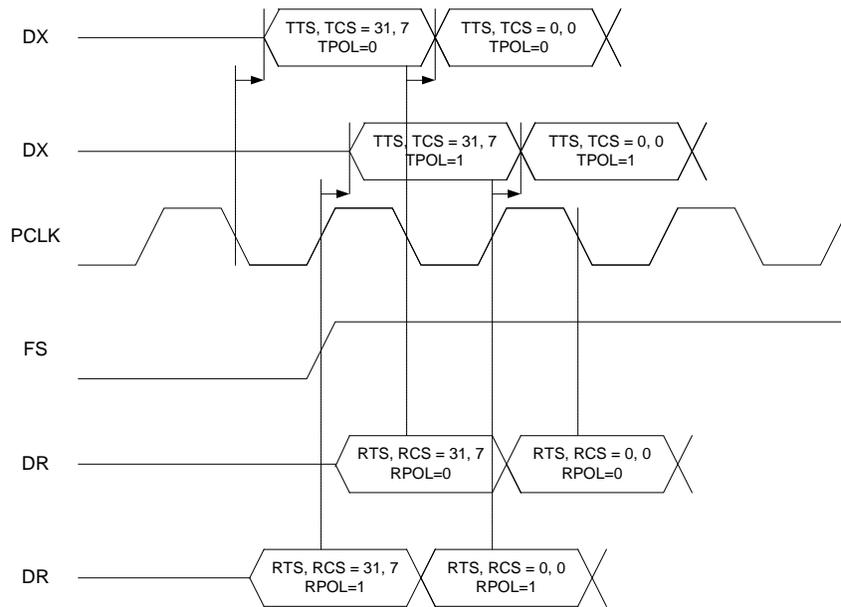
**Figure 1: 73M1866B/73M1966B PCM Frame Bit Numbering**
