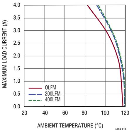
**Figure 16. 5V to 1V<sub>OUT</sub> Derating Curve with BGA Heat Sink**
