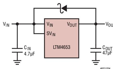
Figure 4. Schottky Diode from  $V_{OUT}$  to  $V_{IN}$
