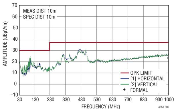
Figure 6. Radiated Emissions Scan of the LTM4653 Producing 24V<sub>OUT</sub> at 4A, from 29.5V<sub>IN</sub>, DC2327A Hardware,  $f_{SW} = 1.2\text{MHz}$ , Measured in a 10m Chamber, Peak Detect Method
