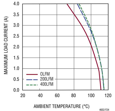
**Figure 24. 48V to 5V<sub>OUT</sub> Derating Curve with BGA Heat Sink**
