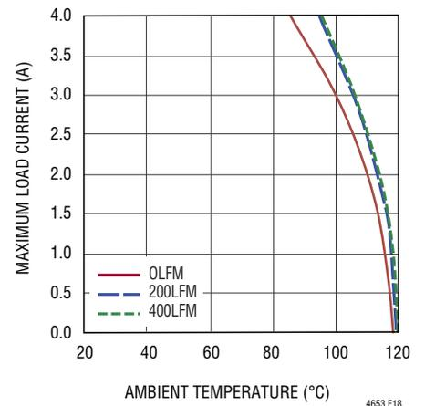
**Figure 18. 24V to 1V<sub>OUT</sub> Derating Curve with BGA Heat Sink**
