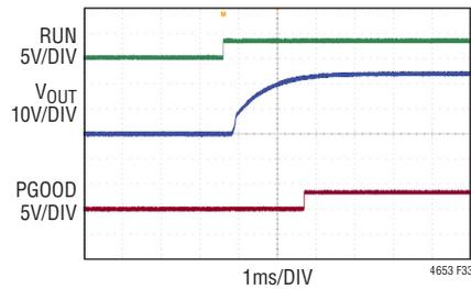
Figure 33. Start-Up Waveforms at 48V<sub>IN</sub>, Figure 32 Circuit
