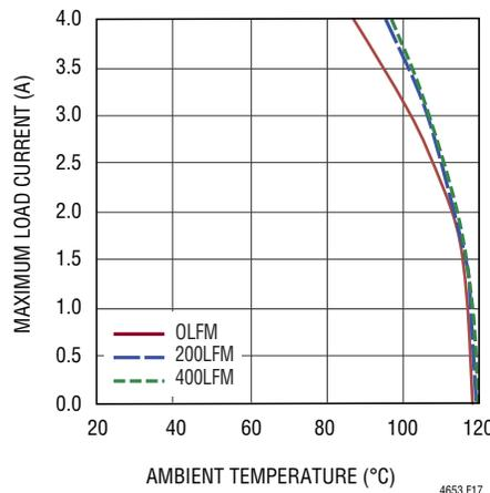
**Figure 17. 12V to 1V<sub>OUT</sub> Derating Curve with BGA Heat Sink**
