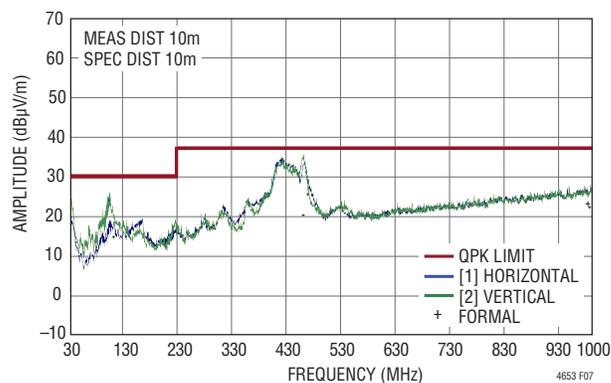
Figure 7. Radiated Emissions Scan of the LTM4653 Producing 24V<sub>OUT</sub> at 3.5A, from 48V<sub>IN</sub>, DC2327A Hardware,  $f_{SW} = 1.2\text{MHz}$ , Measured in a 10m Chamber, Peak Detect Method
