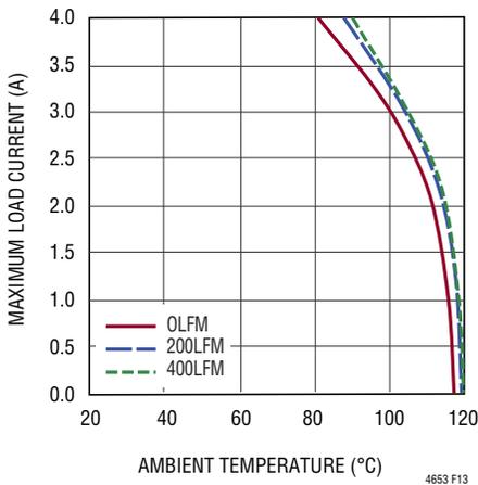
**Figure 13. 5V to 1V<sub>OUT</sub> Derating Curve, No Heat Sink**
