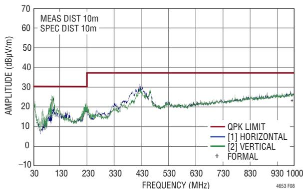
Figure 8. Radiated Emissions Scan of the LTM4653 Producing 12V<sub>OUT</sub> at 3A, from 58V<sub>IN</sub>, DC2327A Hardware,  $f_{SW} = 1.2\text{MHz}$ , Measured in a 10m Chamber, Peak Detect Method
