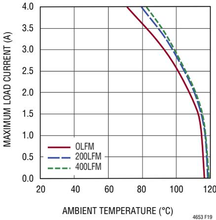
**Figure 19. 12V to 5V<sub>OUT</sub> Derating Curve, No Heat Sink**
