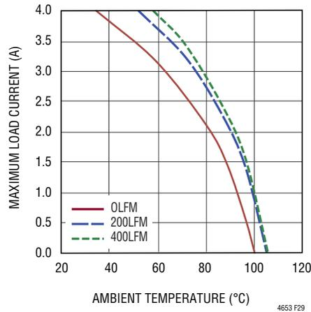
**Figure 29. 48V to 15V<sub>OUT</sub> Derating Curve with BGA Heat Sink**
