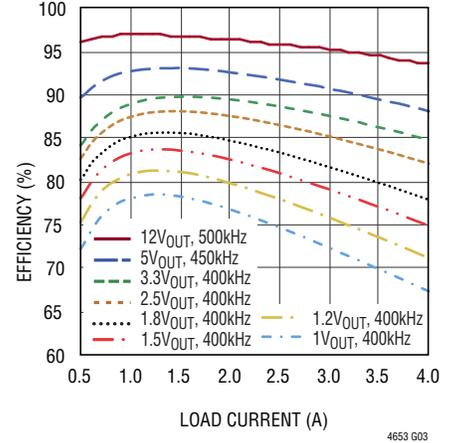
**Efficiency vs Load Current at  $24V_{IN}$ , Forced Continuous Mode**
