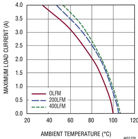
**Figure 26. 48V to 15V<sub>OUT</sub> Derating Curve, No Heat Sink**
