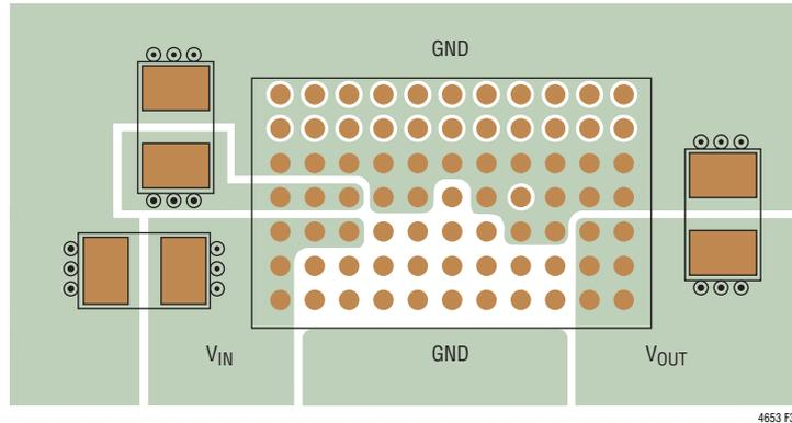
Figure 31. Recommend PCB Layout, Package Top View
