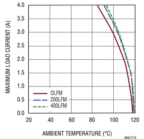
**Figure 15. 24V to 1V<sub>OUT</sub> Derating Curve, No Heat Sink**
