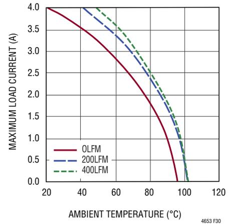
**Figure 30. 48V to 24V<sub>OUT</sub> Derating Curve with BGA Heat Sink**
