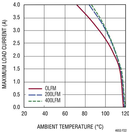
**Figure 22. 12V to 5V<sub>OUT</sub> Derating Curve with BGA Heat Sink**
