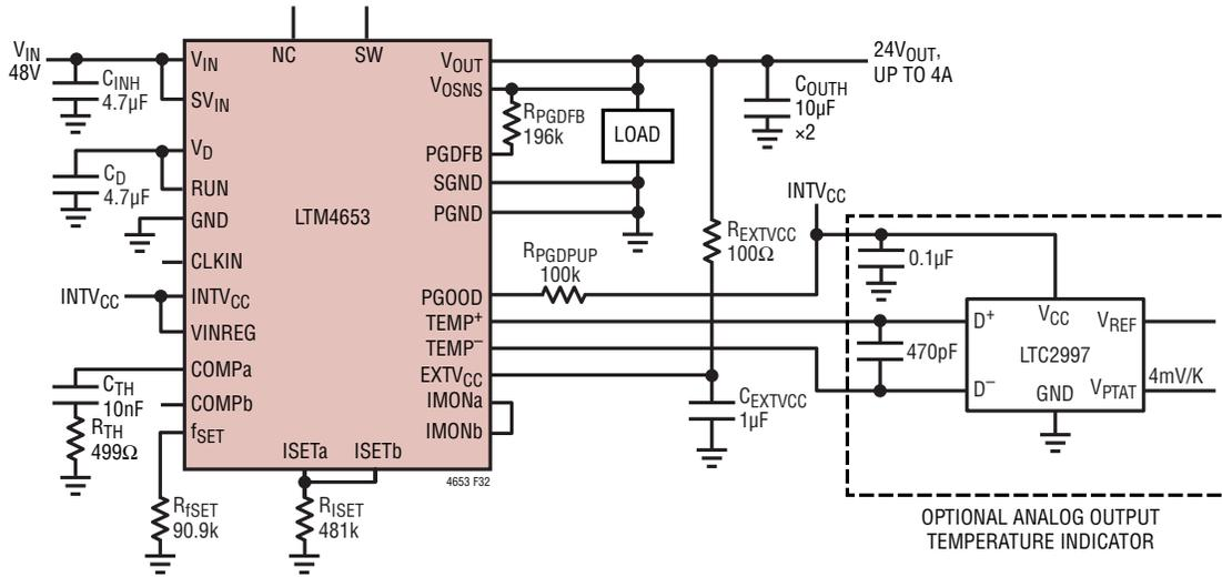
Figure 32. 4A, 24V Output DC/DC μModule Regulator
