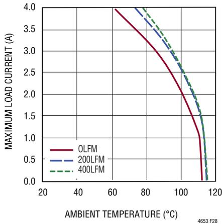
**Figure 28. 24V to 15V<sub>OUT</sub> Derating Curve with BGA Heat Sink**
