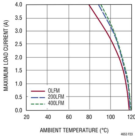
**Figure 23. 24V to 5V<sub>OUT</sub> Derating Curve with BGA Heat Sink**
