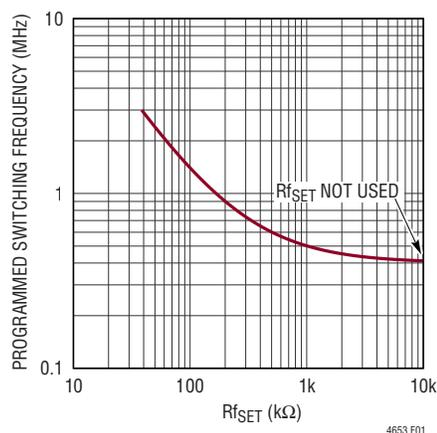
Figure 1. Relationship Between  $R_{\text{fSET}}$  and Target  $f_{\text{sw}}$
