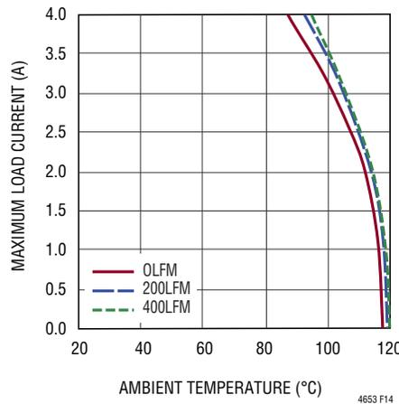
**Figure 14. 12V to 1V<sub>OUT</sub> Derating Curve, No Heat Sink**
