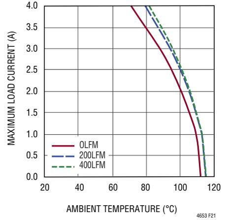
**Figure 21. 48V to 5V<sub>OUT</sub> Derating Curve, No Heat Sink**
