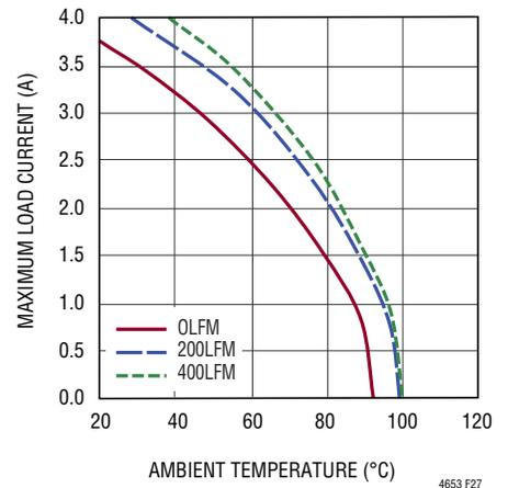
**Figure 27. 48V to 24V<sub>OUT</sub> Derating Curve, No Heat Sink**
