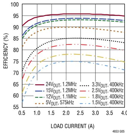
**Efficiency vs Load Current at  $48V_{IN}$ , Forced Continuous Mode**
