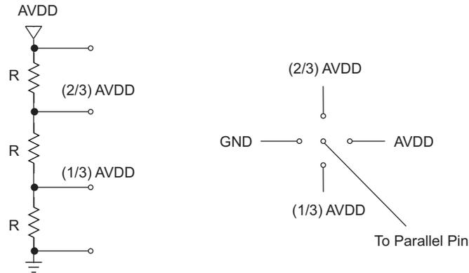
**Figure 4. Simple Scheme to Configure Parallel Pins**
