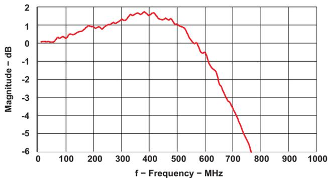
Figure 40. Analog Input Bandwidth, TFADC (Actual Silicon Data)
