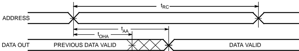
Figure 6. Read Cycle No. 2:  $\overline{OE}$  Controlled [22, 23]
