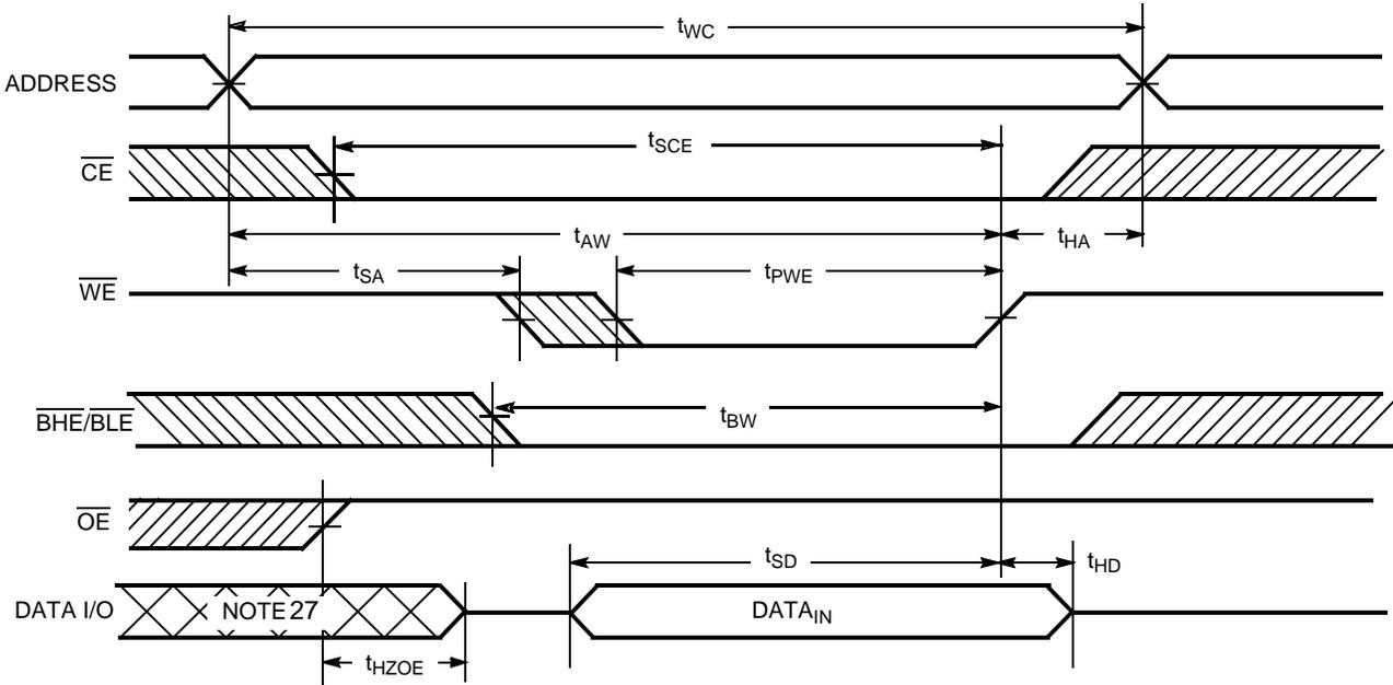
Figure 8. Write Cycle No. 2:  $\overline{CE}$  Controlled [24, 25, 26]
