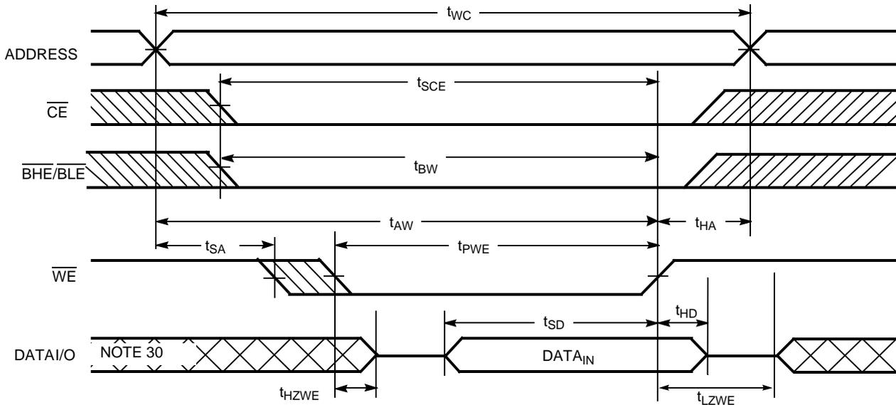
Figure 10. Write Cycle No. 4:  $\overline{BHE/BLE}$  Controlled,  $\overline{OE}$  LOW [28]
