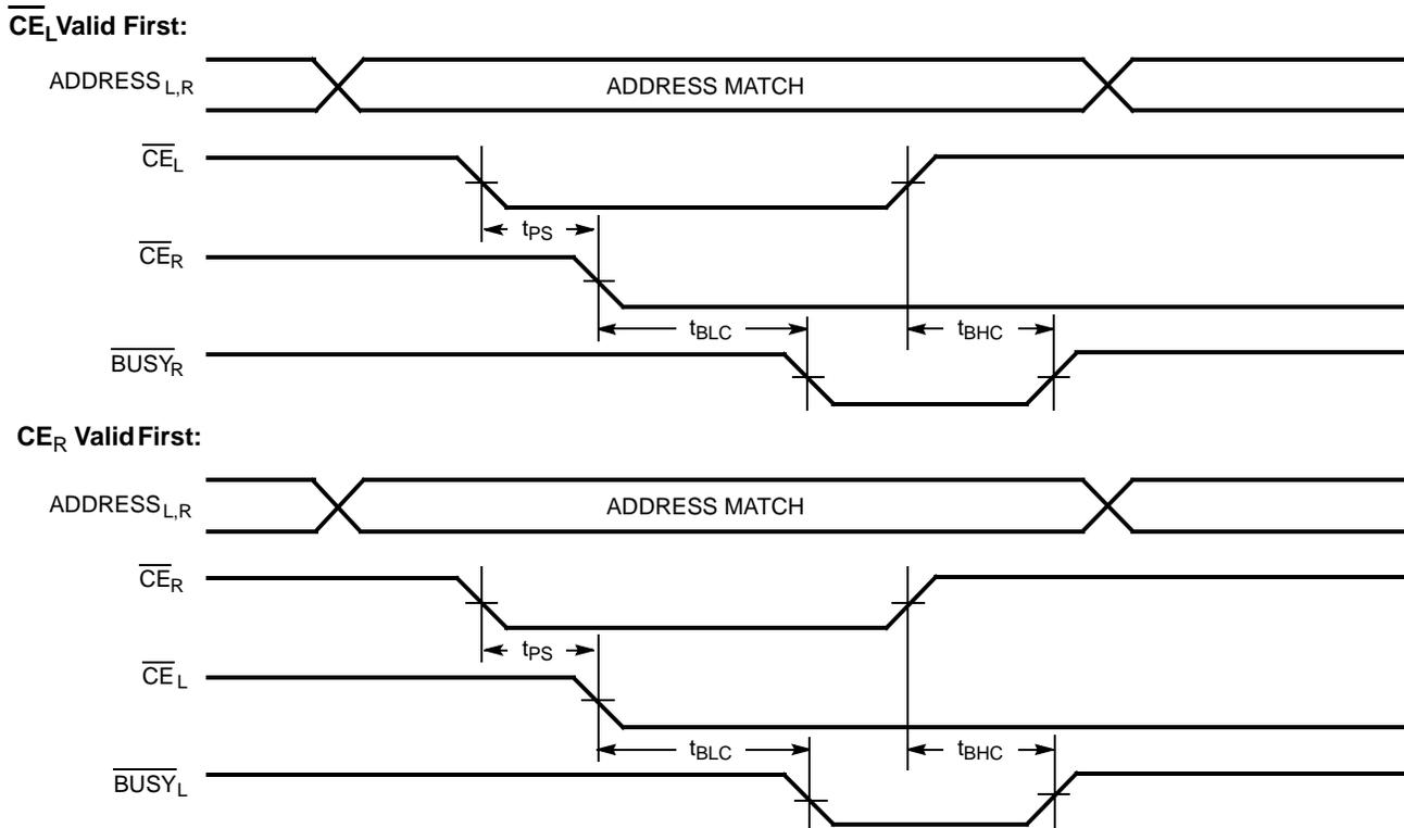
Figure 14. Busy Timing Diagram No. 2 (Address Arbitration) [49]
