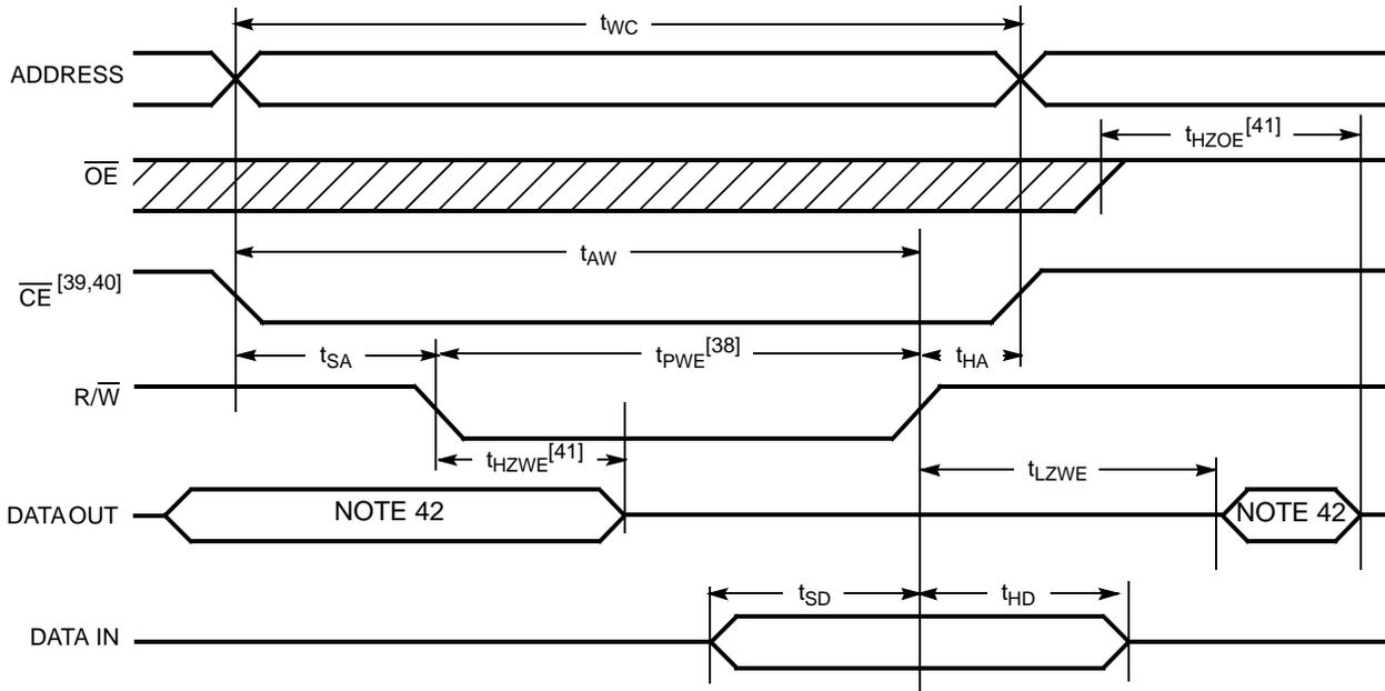
Figure 8. Write Cycle No. 2 (CE Controlled Timing) [35, 36, 37, 43]
