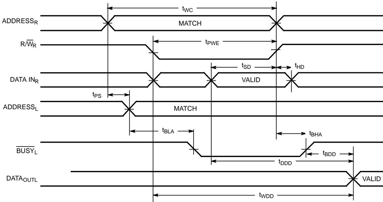
Figure 12. Write Timing with Busy Input ( $\overline{\text{M/S}} = \text{LOW}$ )
