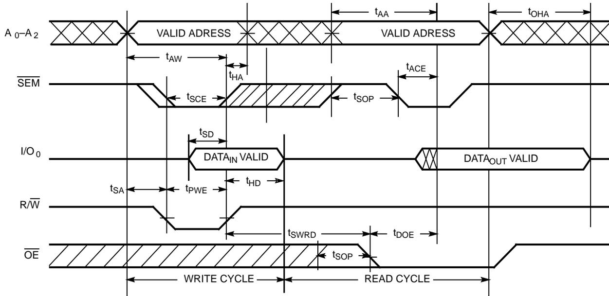
Figure 10. Timing Diagram of Semaphore Contention [45, 46, 47]
