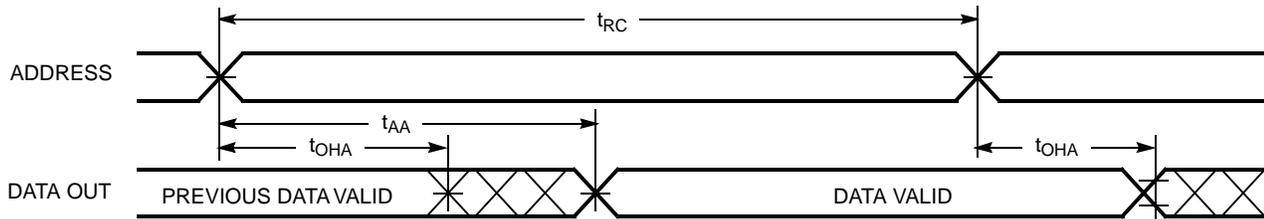
Figure 5. Read Cycle No. 2 (Either Port  $\overline{CE}/\overline{OE}$  Access) [30, 33, 34]
