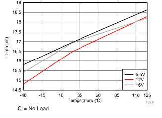
Figure 23. LO Falling Propagation Delay (TDLFF)
