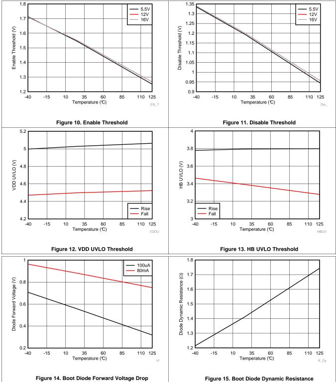
Figure 15. Boot Diode Dynamic Resistance
