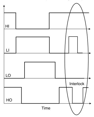
Figure 24. Interlock or Input Shoot-through Protection
