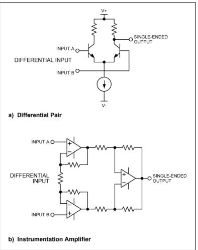
Figure 5. These differential-amplifier circuits exhibit high common-mode rejection.
