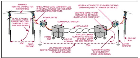
Figure 1. This generalized system transmits data between two widely separated buildings, and shows the earth currents created between ground points in a single-phase power-distribution system. Similar currents are created in 3-phase, Y-connected systems.
