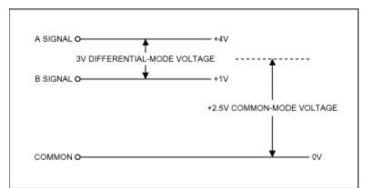
Figure 3. Typical RS-485 transmitters generate a common-mode DC offset voltage as shown.
