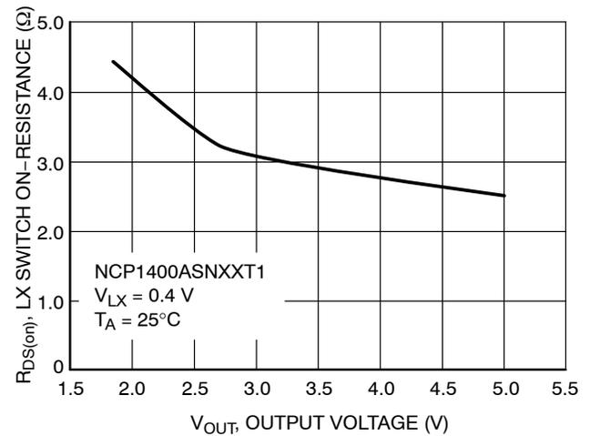
**Figure 25. NCP1400ASNXXT1 LX Switch On-Resistance vs. Output Voltage**
