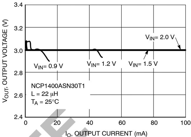
**Figure 3. NCP1400ASN30T1 Output Voltage vs. Output Current**
