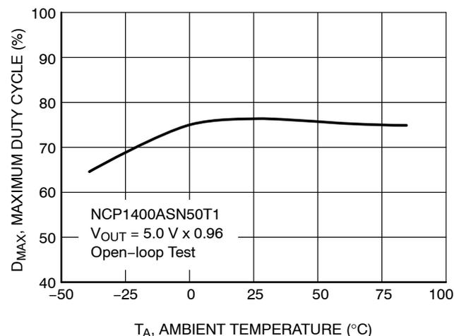
Figure 19. NCP1400ASN50T1 Maximum Duty Cycle vs. Temperature
