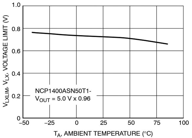
**Figure 13. NCP1400ASN50T1  $V_{LX}$  Voltage Limit vs. Temperature**
