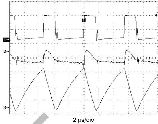
$V_{OUT} = 3.0\text{ V}$ ,  $V_{IN} = 1.2\text{ V}$ ,  $I_O = 25\text{ mA}$ ,  $L = 22\text{ }\mu\text{H}$ ,  $C_{OUT} = 68\text{ }\mu\text{F}$
