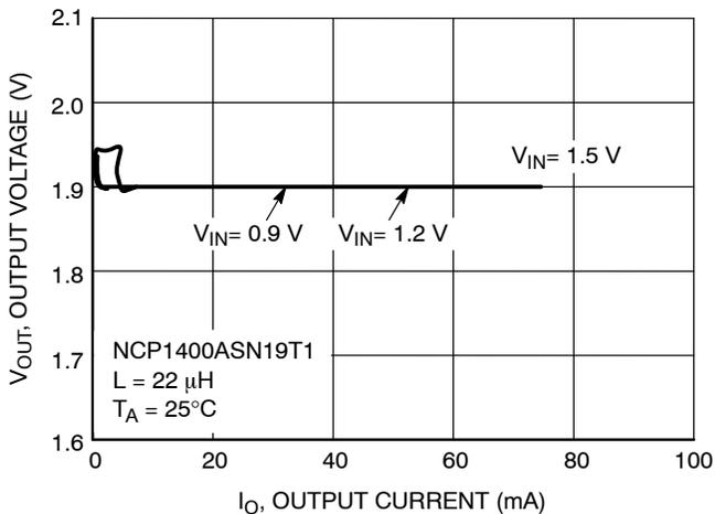
**Figure 2. NCP1400ASN19T1 Output Voltage vs. Output Current**
