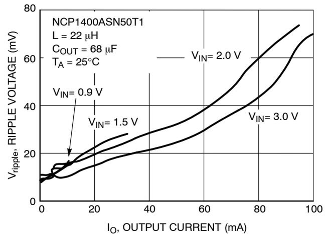
**Figure 31. NCP1400ASN50T1 Ripple Voltage vs. Output Current**
