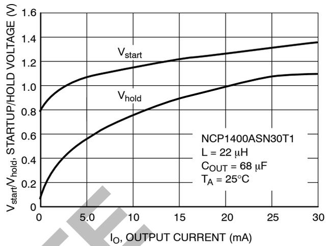
**Figure 27. NCP1400ASN30T1 Operation Startup/Hold Voltage vs. Output Current**
