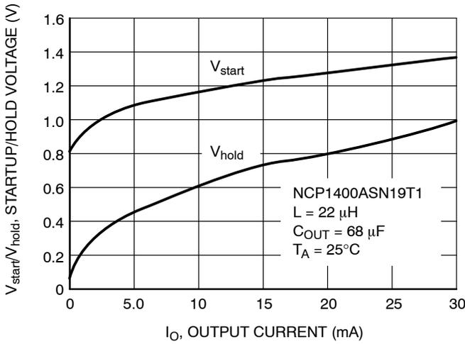
**Figure 26. NCP1400ASN19T1 Operation Startup/Hold Voltage vs. Output Current**
