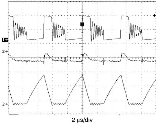
$V_{OUT} = 3.0\text{ V}$ ,  $V_{IN} = 1.2\text{ V}$ ,  $I_O = 10\text{ mA}$ ,  $L = 22\text{ }\mu\text{H}$ ,  $C_{OUT} = 68\text{ }\mu\text{F}$
