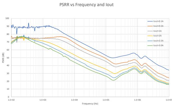
$V_{IN}=1.1\text{V}$ ,  $V_{out}=0.8\text{V}$ ,  $V_{BIAS}=5\text{V}$ ,  $C_{OUT}=(47+10+10)\mu\text{F}$ ,  $C_{SS}=10\text{nF}$ ,  $C_{FF}=10\text{nF}$
