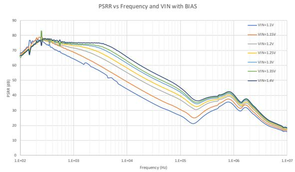
$V_{out}=0.8\text{V}$ ,  $V_{BIAS}=5\text{V}$ ,  $I_{out}=3\text{A}$ ,  $C_{OUT}=(47+10+10)\mu\text{F}$ ,  $C_{SS}=10\text{nF}$ ,  $C_{FF}=10\text{nF}$
