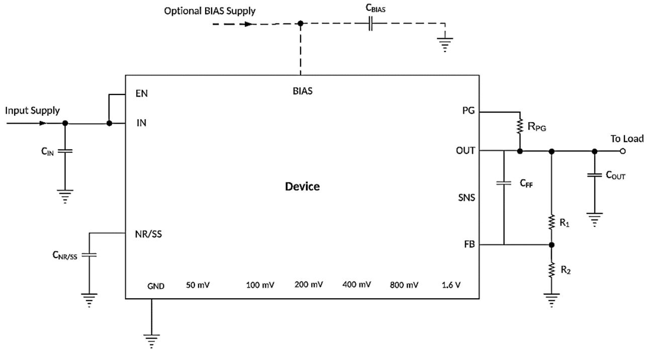
Figure 10 Adjustable Operation
