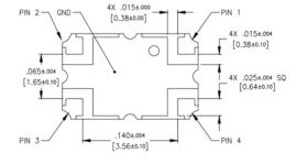
Dimensions are in Inches [Millimeters] X3C19F1-03S Mechanical Outline
