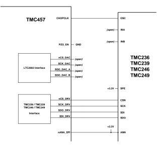
Figure 4 : Stepper Motor Driver Configuration (SPI)
