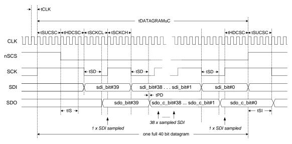
Figure 8 : Timing Diagram of the Serial Micro Controller Interface
