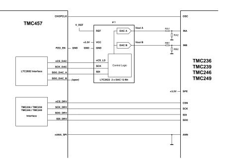
Figure 3 : High Resolution Micro Stepping Configuration
