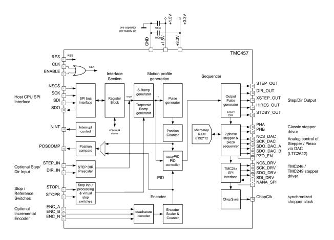
Figure 1 : Functional Block Diagram of the TMC457
