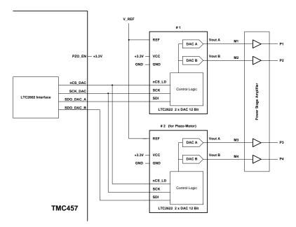
Figure 2 : TMC457 with Piezo Motor Interface
