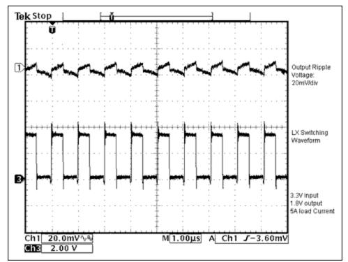
Figure 2. Output ripple voltage and LX switching waveforms.
