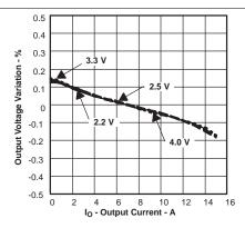
Figure 26. Load Regulation vs Output Current
