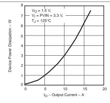
Figure 6. Device Power Dissipation vs Output Current
