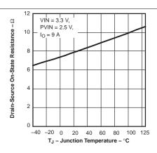
Figure 2. Drain-Source On-State Resistance vs Junction Temperature
