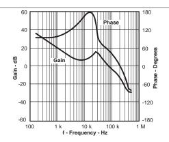
Figure 25. Measured Loop Response vs Frequency
