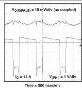
Figure 30. Output Voltage Ripple
