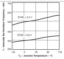
Figure 3. Internally Set Oscillator Frequency vs Junction Temperature
