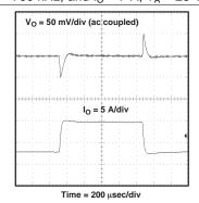
Figure 21. Load Transient Response
