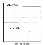
Figure 23. Start-Up Waveform Output Voltage Relative To VIN
