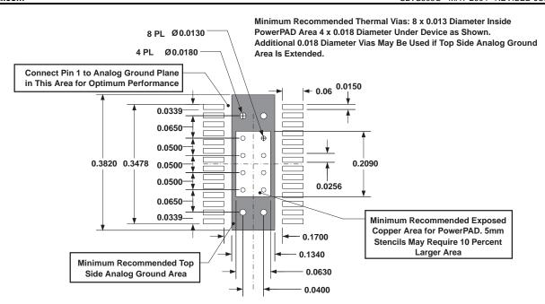
Figure 34. Recommended Land Pattern for 28-Pin PWP PowerPAD
