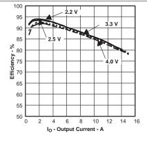
Figure 28. Efficiency vs Output Current
