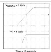
Figure 22. Start-Up Waveform Output Voltage Relative To Enable
