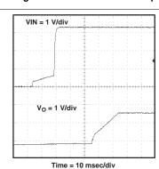
Figure 33. Start-Up Waveform Output Voltage Relative to Enable
