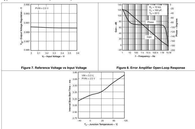
Figure 9. Internal Slow-Start Time vs Junction Temperature
