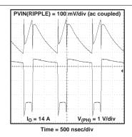
Figure 29. Input Ripple Voltage
