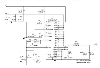
Figure 11. Application Circuit, 2.5 V to 1.5 V
