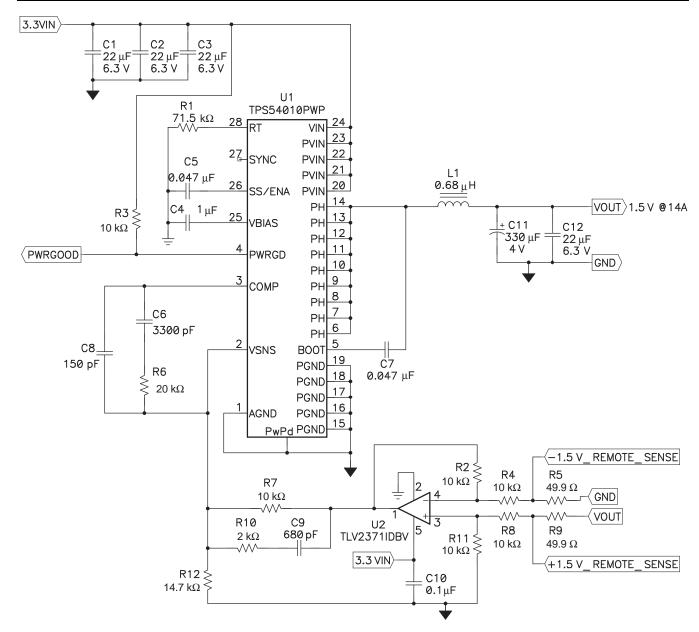
Figure 13. 1.5-V Power Supply With Remote Sense
