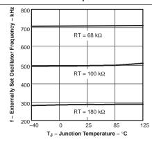
Figure 4. Externally Set Oscillator Frequency vs Junction Temperature
