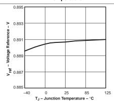
Figure 5. Voltage Reference vs Junction Temperature
