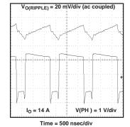
Figure 19. Input Ripple Voltage
