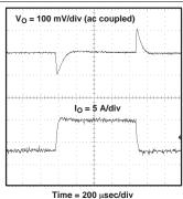
Figure 31. Load Transient Response
