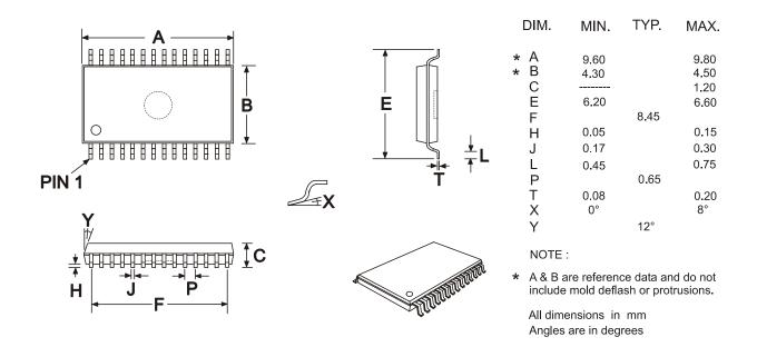
Figure 17 Mechanical Outline of 28-pin TSSOP (E1): Order as part no. CMX882E1
