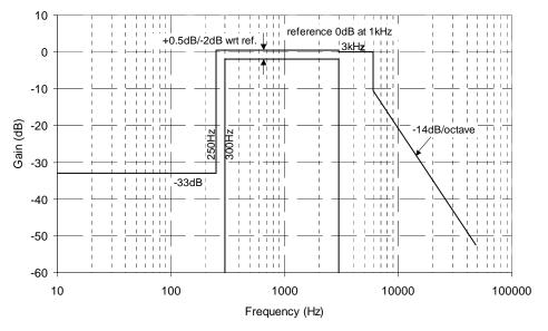
Figure 8 25kHz Channel Audio Filter Response Template
