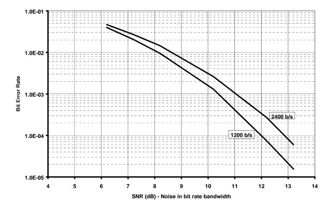
Figure 15 Typical FFSK/MSK Bit Error Rate Graph
