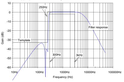
Figure 5 Rx Audio Filter Frequency Response
