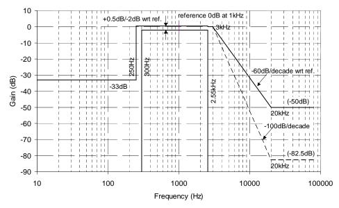
Figure 9 12.5kHz Channel Audio Filter Response Template
