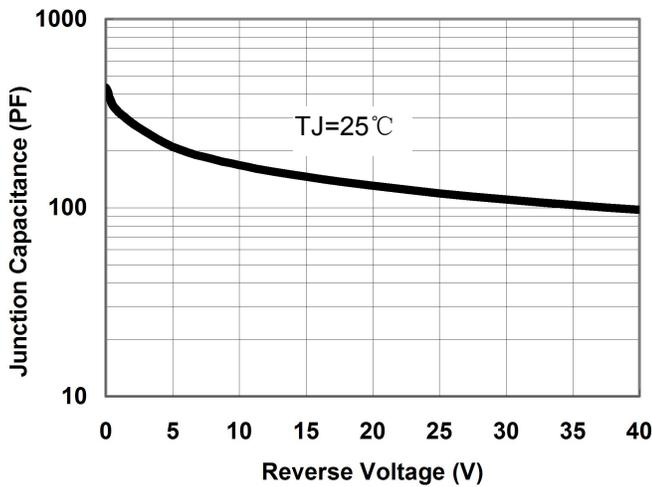
Fig.1-Typical Junction Capacitance
