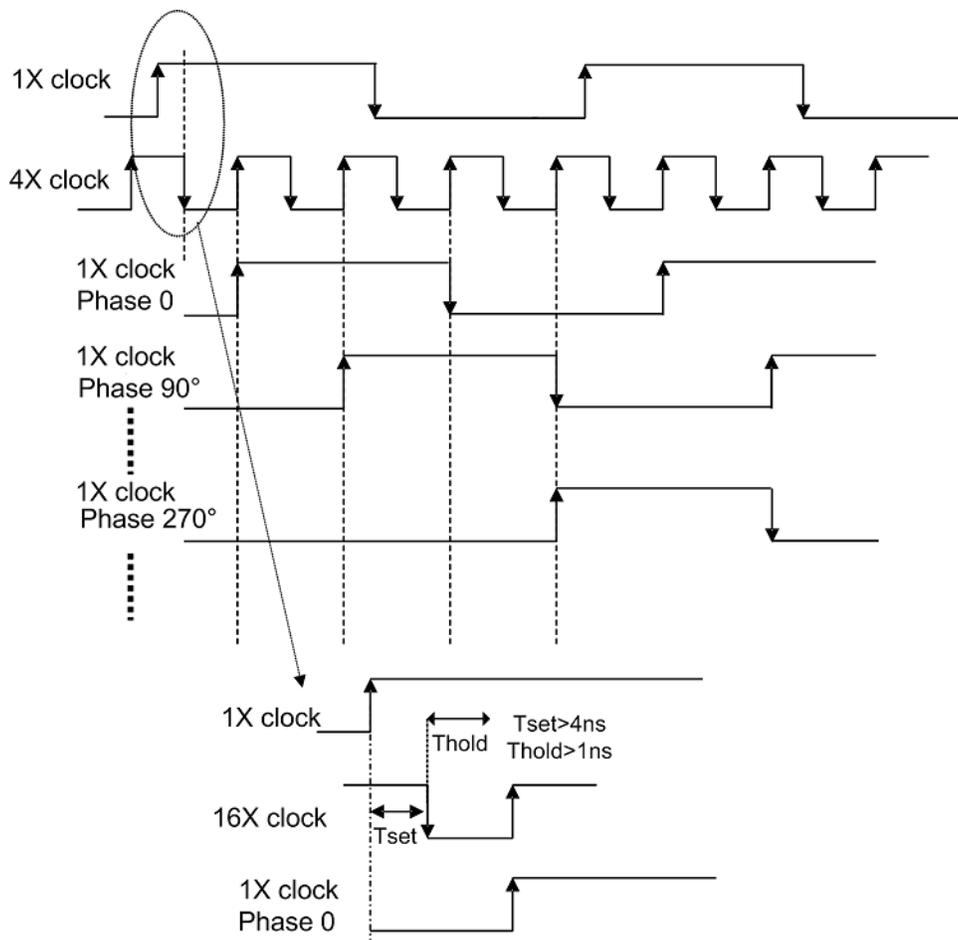
Figure 75.  $8 \times f_{cw}$  and  $4 \times f_{cw}$  Timing Diagram
