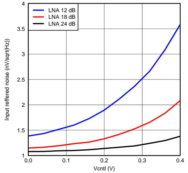
Figure 23. IRN, PGA = 24dB and Low Power Mode
