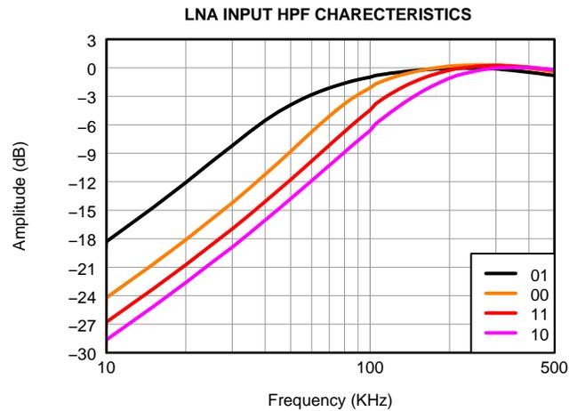
**Figure 13. LNA High-Pass Filter Response vs. Reg59[3:2]**
