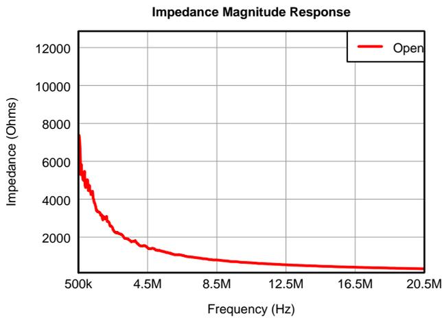
Figure 8. Input Impedance without Active Termination (Magnitude)
