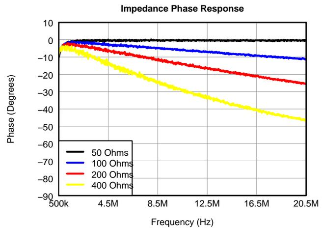
Figure 11. Input Impedance with Active Termination (Phase)
