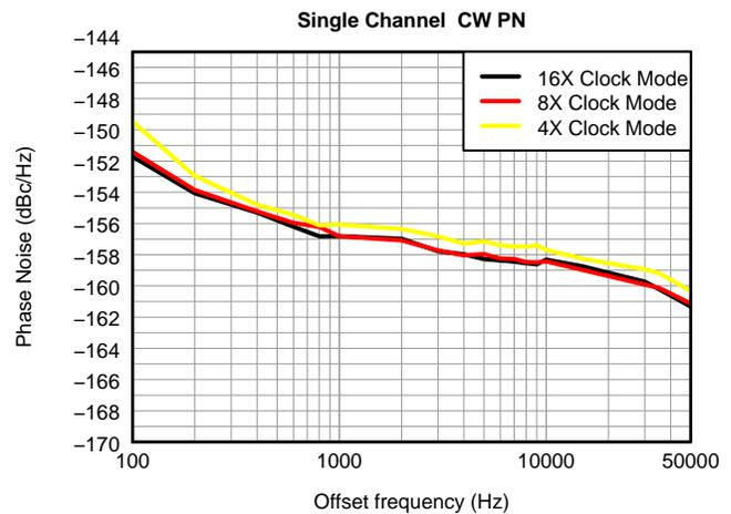
**Figure 15. CW Phase Noise, Fin = 2MHz**
