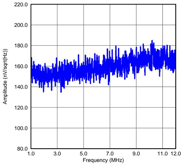
Figure 28. ORN, PGA = 24dB and Low Power Mode
