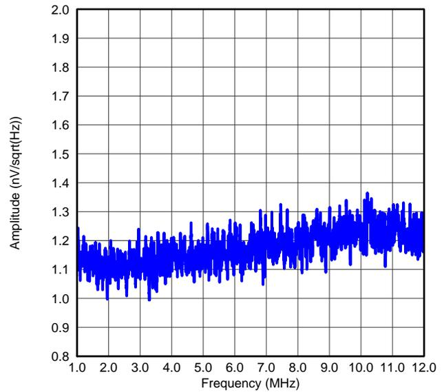
Figure 27. IRN, PGA = 24dB and Low Power Mode
