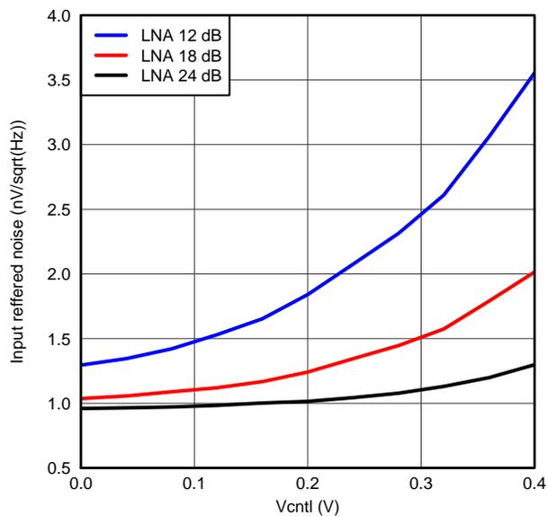
Figure 21. IRN, PGA = 24dB and Medium Power Mode
