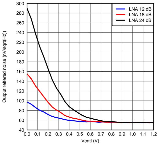
Figure 26. ORN, PGA = 24 dB and Low Power Mode
