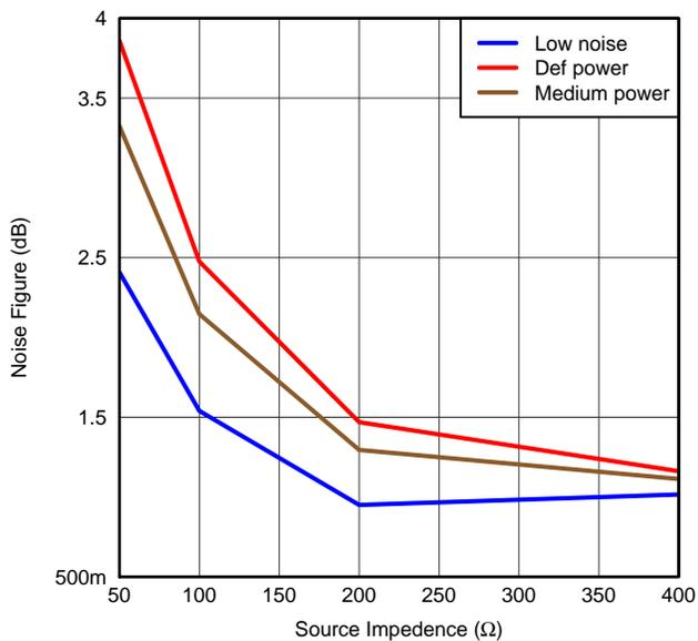
Figure 36. Noise Figure vs. Power Modes without Termination
