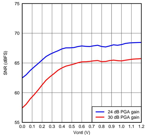
Figure 29. SNR, LNA = 18dB and Low Noise Mode
