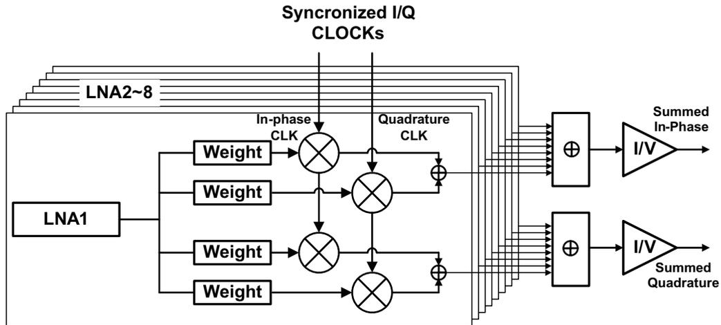
Figure 76. Block Diagram of  $1 \times f_{cw}$  mode
