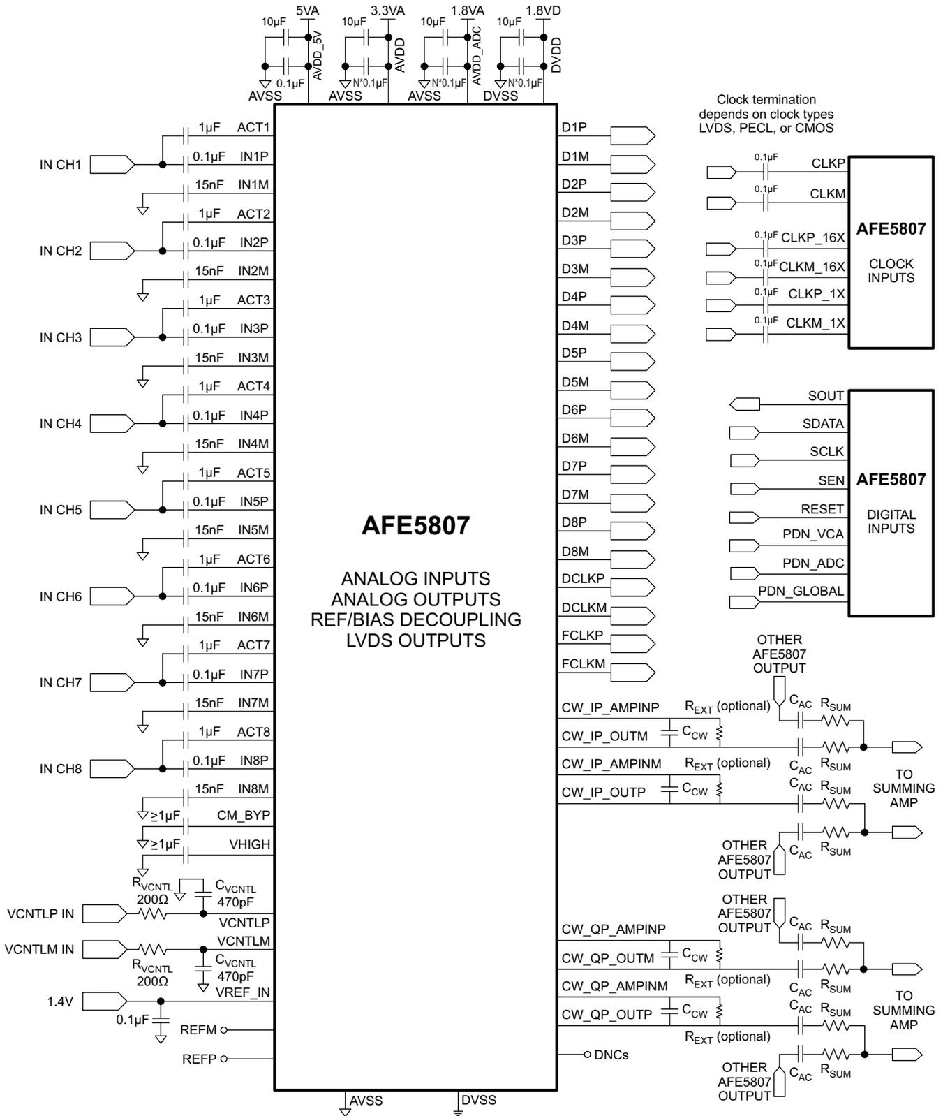
Figure 82. Application Circuit
