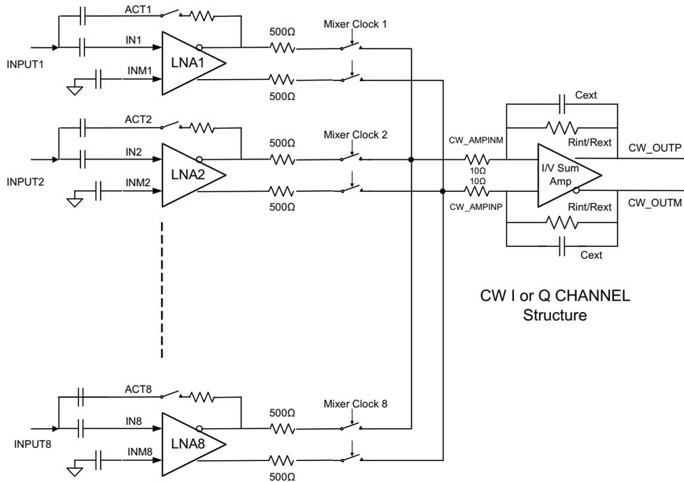
Note: the 10~15 Ω parasitic resistors at CW\_AMPINM/P are due to internal IC routing and can create slight attenuation.
