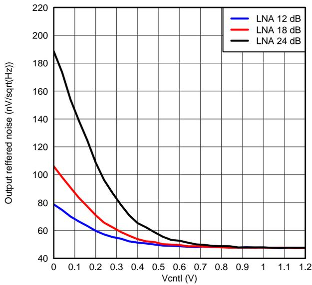
Figure 24. ORN, PGA = 24dB and Low Noise Mode
