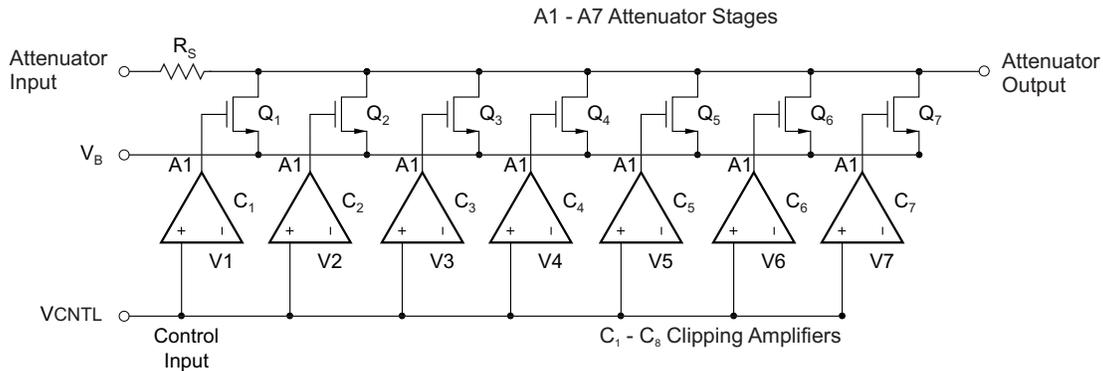
**Figure 66. Simplified Voltage Controlled Attenuator (Analog Structure)**
