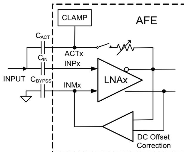
Figure 65. AFE5807 LNA with DC Offset Correction Circuit
