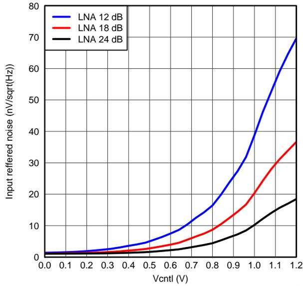
Figure 22. IRN, PGA = 24dB and Low Power Mode
