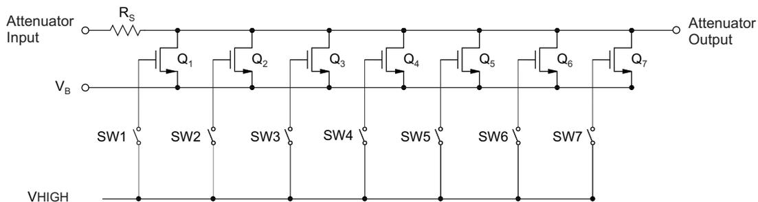
**Figure 67. Simplified Voltage Controlled Attenuator (Digital Structure)**
