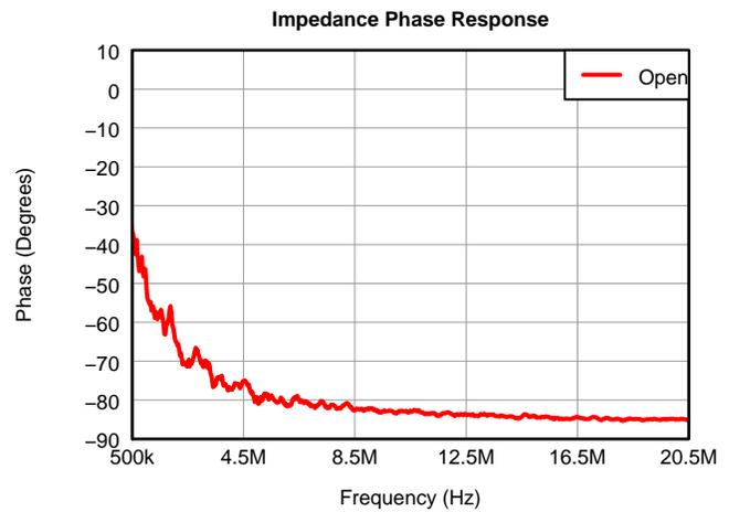
Figure 9. Input Impedance without Active Termination (Phase)
