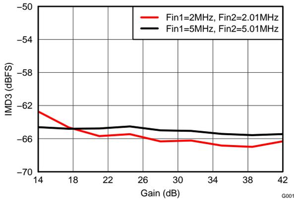
Figure 46. IMD3, Fout1 = -7dBFS and Fout2 = -7dBFS
