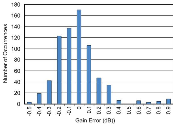
Figure 6. Gain Matching Histogram,  $V_{CNTL} = 0.9V$  (936 Channels)
