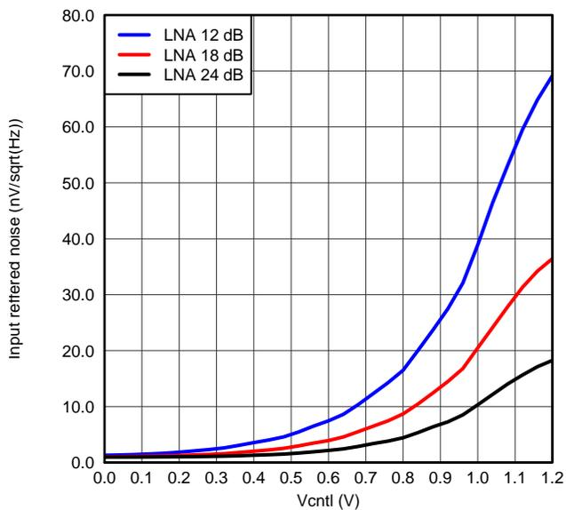
Figure 20. IRN, PGA = 24dB and Medium Power Mode
