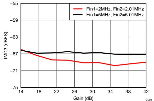
Figure 45. IMD3,  $F_{out1} = -7dBFS$  and  $F_{out2} = -21dBFS$
