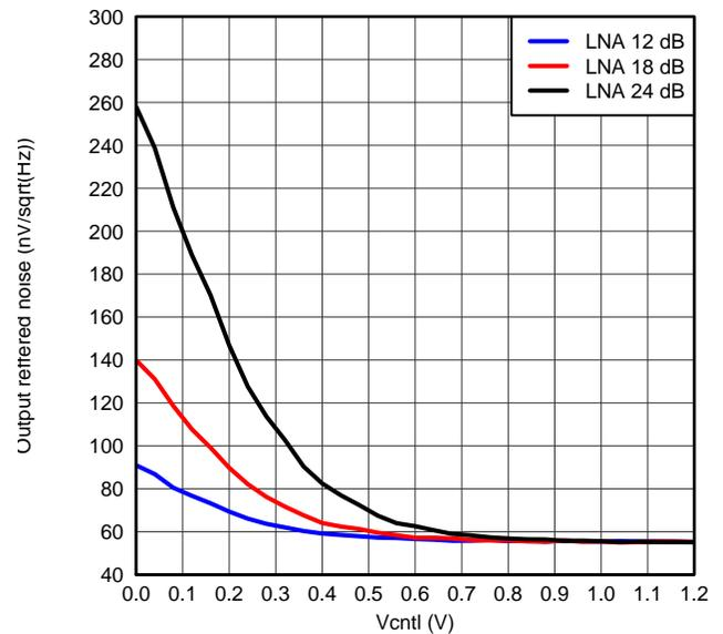
Figure 25. ORN, PGA = 24 dB and Medium Power Mode
