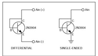
*Figure 1. Connecting differential and single-ended temperature sensors.*
