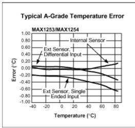
Figure 2. Typical A-grade temperature error.
