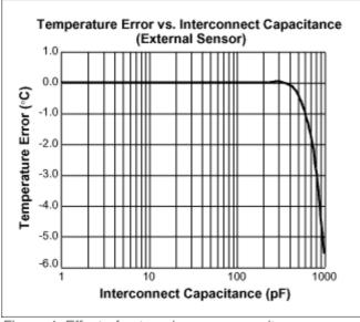
Figure 4. Effect of external sensor capacitance.
