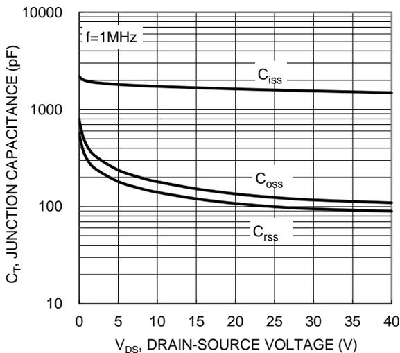
Figure 11. Typical Junction Capacitance
