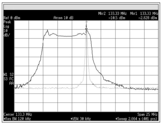
Figure 1. Clock spectrum of the DS4M133 with MS = low and MS = 8kHz (low to  $V_{CC}/2$ ) downspreading.
