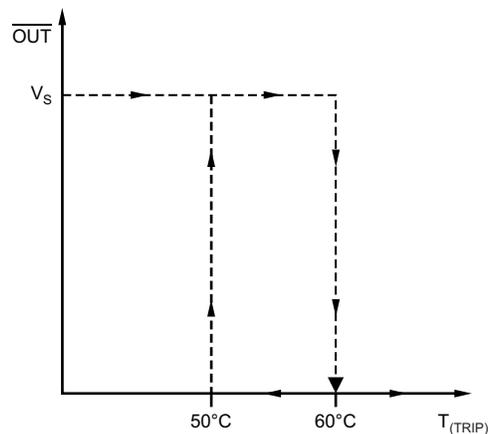
**Figure 9. TMP302A-Q1: HYSTSET =  $V_S$ , TRIPSET1 =  $V_S$ , TRIPSET0 = GND**
