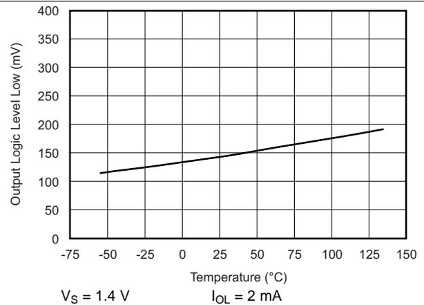
Figure 6. Output Logic-Level Low  $V_{OL}$  vs Temperature
