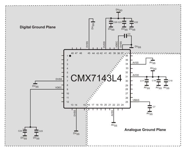
Figure 3 CMX7143 Power Supply and De-coupling
