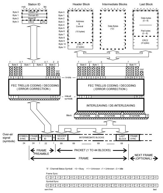
Figure 17 RD-LAP Over Air Signal Format
