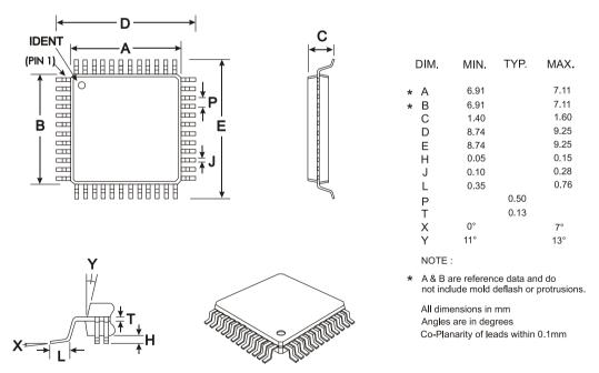
Figure 27 Mechanical Outline of 48-pin LQFP (L4)
