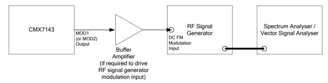
Figure 18 Tx Spectrum and Modulation Measurement Configuration
