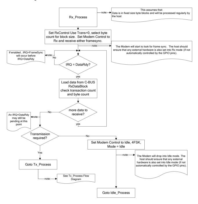
Figure 8 Host Rx Data Flow (Use Trans=0)
