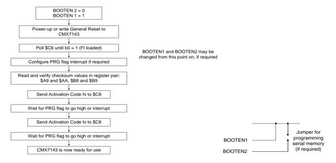
Figure 6 FI Loading from Serial Memory
