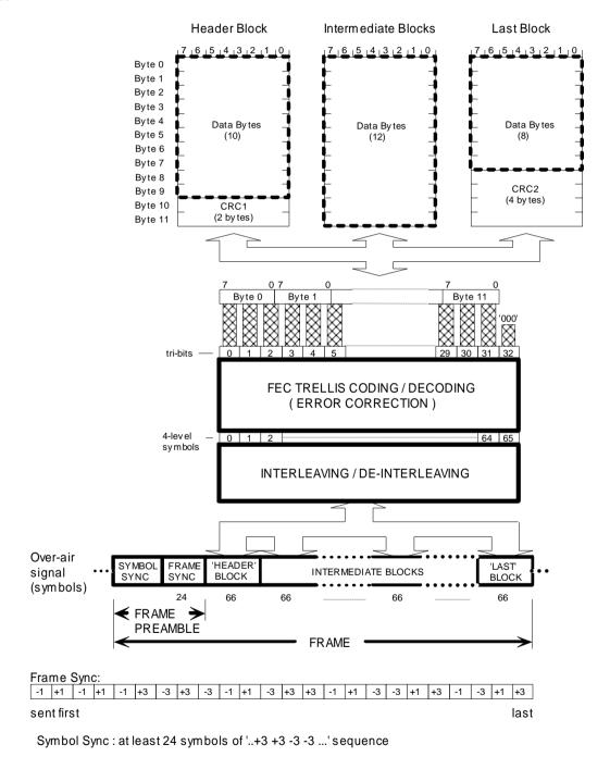
Figure 15 Formatted Data Over Air Signal Format
