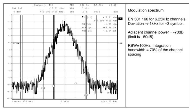
Figure 21 Tx Modulation Spectra (4FSK), 4800bps - 2-point modulation
