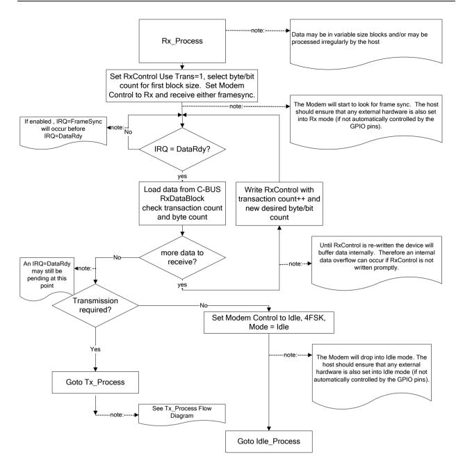
Figure 9 Host Rx Data Flow (Flow controlled data with UseTrans=1)
