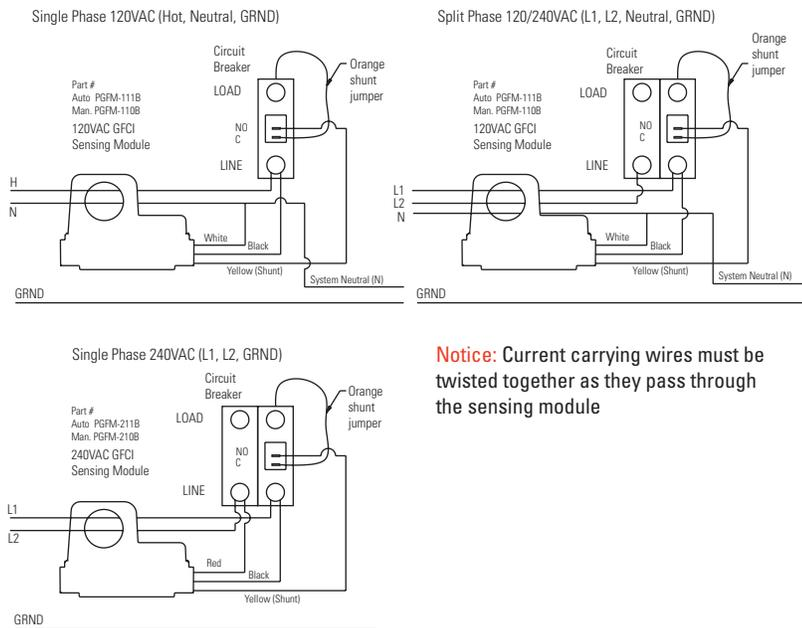
**Notice:** Current carrying wires must be twisted together as they pass through the sensing module
