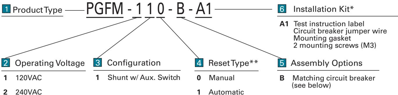
To determine a matching circuit breaker for use in tandem with the LineGard™ Sensing Module, please contact us directly or your local Sensata Representative for assistance with the appropriate identifying part number.
