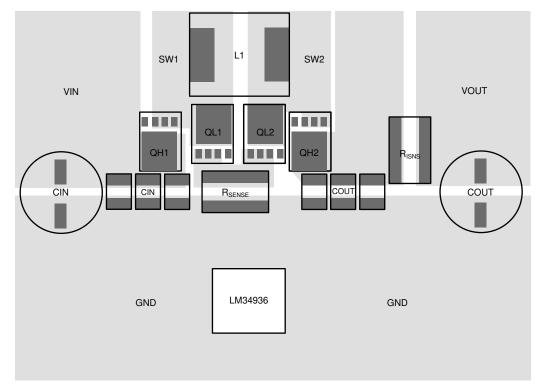
Figure 10-1. LM34936 Power Stage Layout
