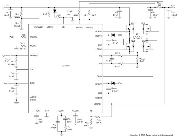
Figure 8-1. LM34936 Four-Switch Buck Boost Application Schematic
