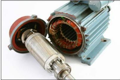
Rotor and stator of an induction motor.
