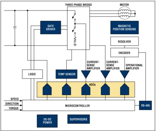
Block diagram of a typical industrial motor control. For a list of Maxim's recommended motor-drive solutions, please go to: www.maximintegrated.com/motordrive.
