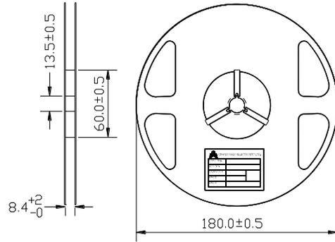
● Dimensions of Tape (Unit: mm)
