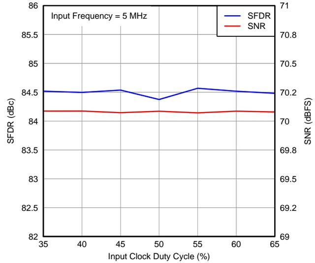
Figure 21. Performance vs. Input Clock Duty Cycle
