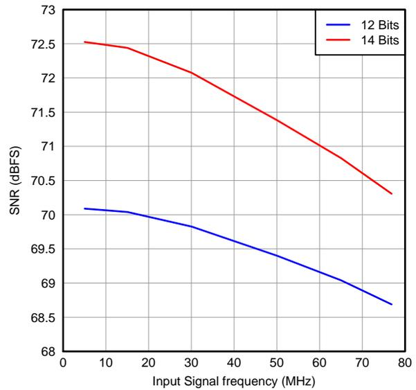
Figure 15. Signal-to-Noise Ratio Across Input Signal Frequency
