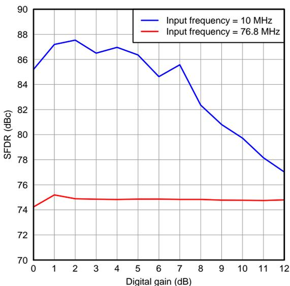
Figure 18. Spurious-Free Dynamic Range vs. Digital Gain
