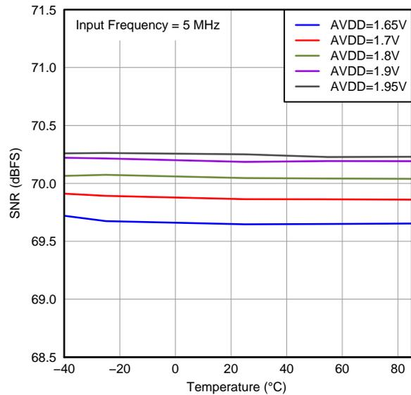
Figure 23. Signal-to-Noise Ratio Across AVDD and Temperature
