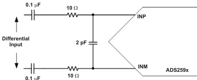
Figure 57. Drive Circuit
