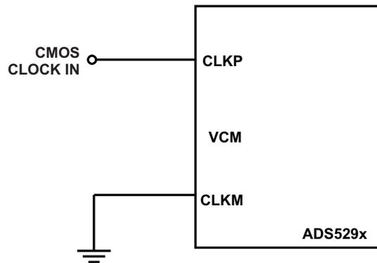
Figure 59. Drive Circuit
