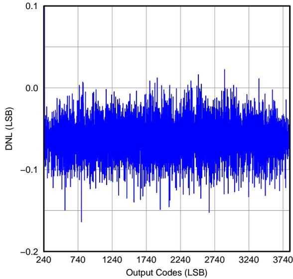
**Figure 28. Differential Non-Linearity**
