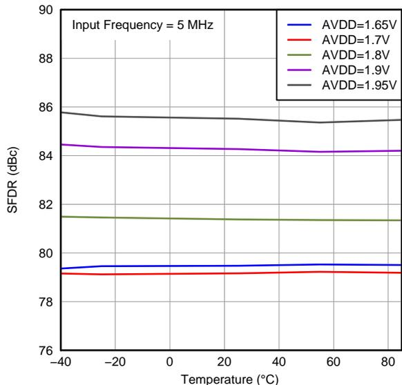
**Figure 24. Spurious-Free Dynamic Range Across AVDD and Temperature**
