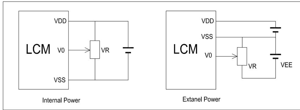
$V_{DD}-V_0$ : LCD Driving voltage
