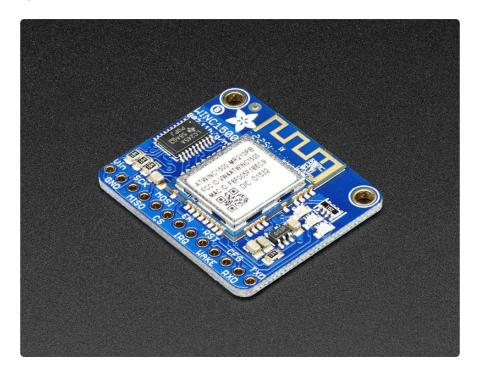
Connect your Arduino to the Internet with this fine new FCC-certified WiFi module from Atmel. This 802.11bgn-capable WiFi module is the best new thing for networking your devices, with SSL support and rock solid performance - running our adafruit.io MQTT demo for a full weekend straight with no hiccups (it would have run longer but we had to go to work, so we unplugged it). We like these so much, they've completely replaced the CC3000 module on all our projects.
