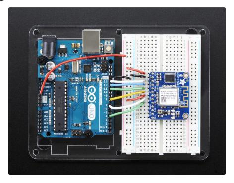
For this initial demo we'll be using an Arduino UNO to connect. You can also use an Arduino Zero, but you'll have to use the ICSP 6-pin header not pins 11,12,13
