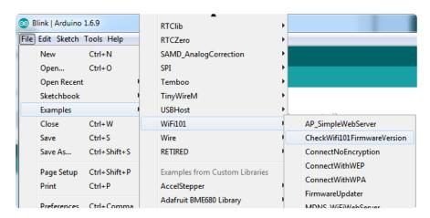
Note that to use the official Arduino WiFi101 Library, we must configure it to use the pins specific to the ATWINC1500 Breakout. With each example sketch, you'll need to add WiFi.setPins(8,7,4); to the top of the setup function, before WiFi.status() is called.
