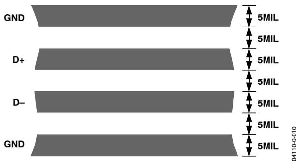
Figure 24. Typical Arrangement of Signal Tracks
