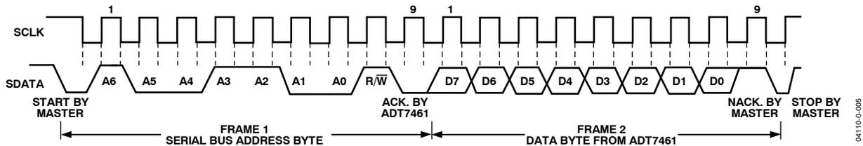
Figure 19. Reading from a Previously Selected Register
