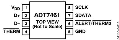
Figure 3. Pin Configuration
