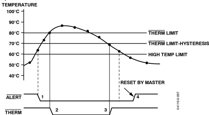
Figure 21. Operation of the  $\overline{\text{ALERT}}$  and  $\overline{\text{THERM}}$  Interrupts
