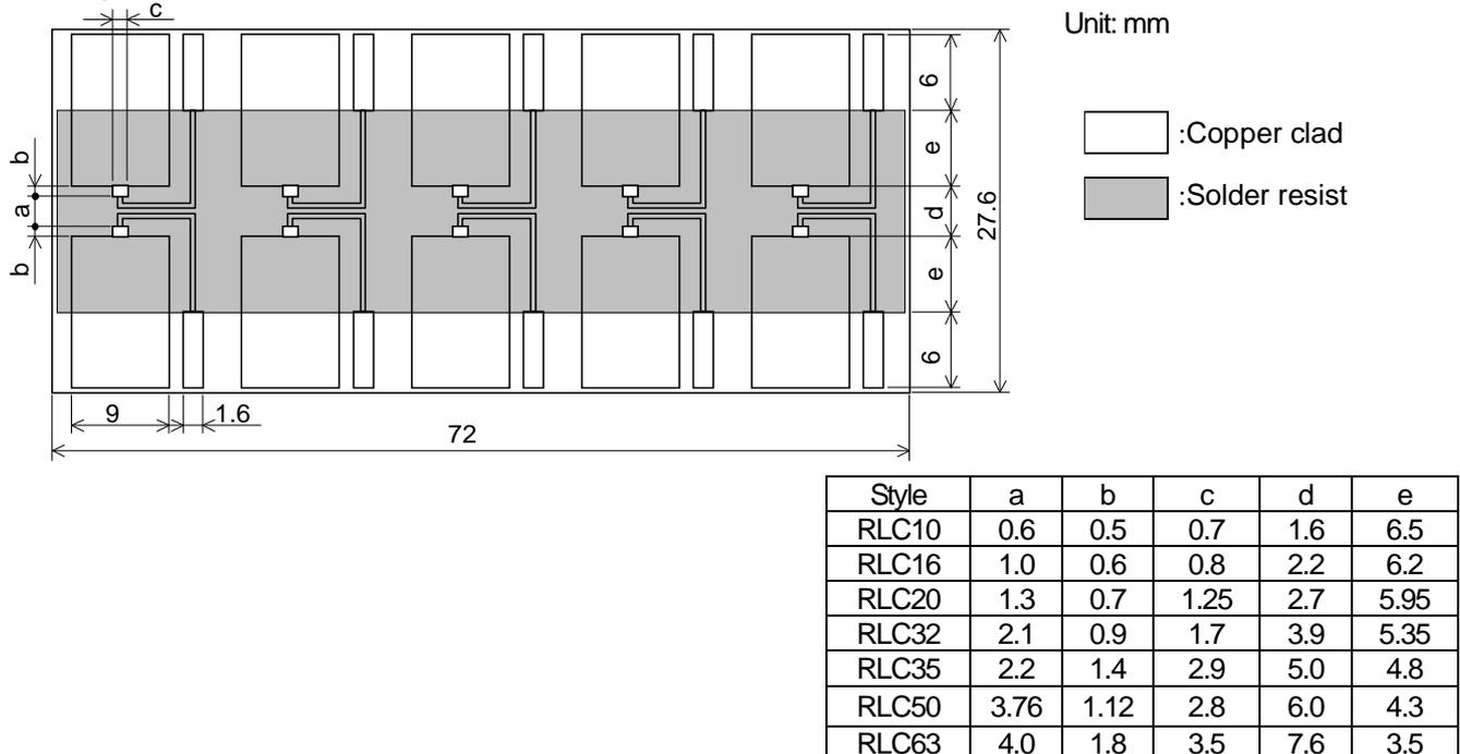
Figure-3 RLC TEST SUBSTRATE
