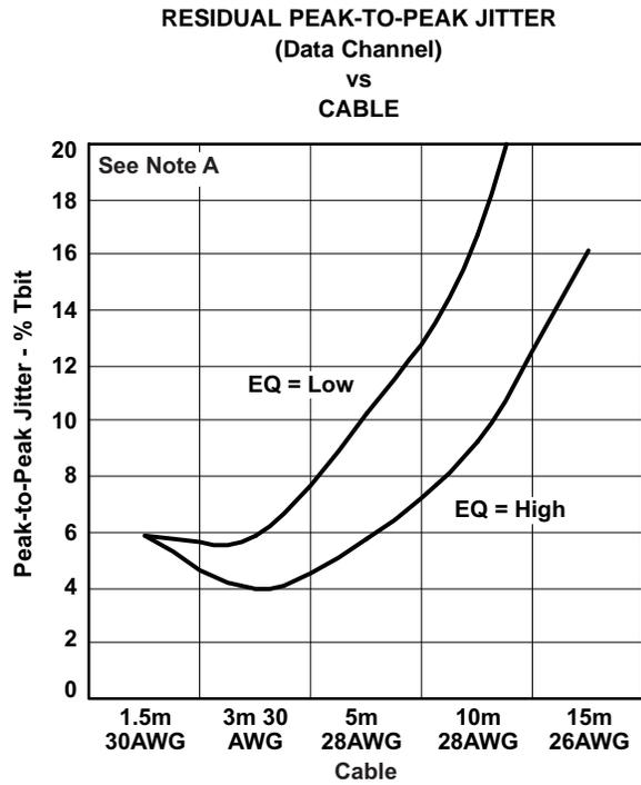
A. 1080p 10-Bit,  $V_{CC} = AV_{CC} = 3.3\text{ V}$ ,  $T_A = 25^\circ\text{C}$ ,  $R_{VSADJ} = 4.02\text{ k}\Omega$ , See Figure 6, Clock Channel = 185.6 MHz, Data Channel = 1.856 Gbps
