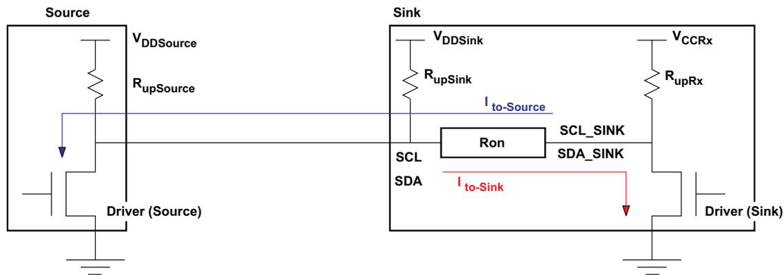
Figure 17. Simplified Electrical Circuit Model for DDC Channel
