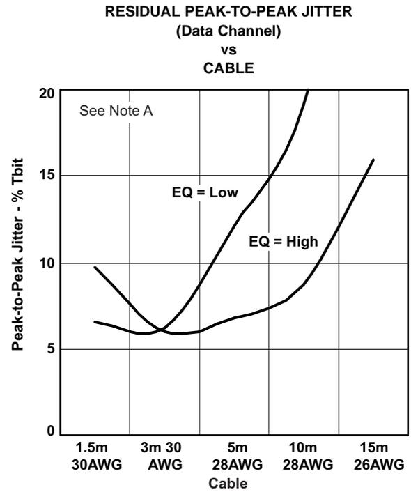
A. 1080p 12-Bit,  $V_{CC} = AV_{CC} = 3.3\text{ V}$ ,  $T_A = 25^\circ\text{C}$ ,  $R_{VSADJ} = 4.02\text{ k}\Omega$ , See Figure 6, Clock Channel = 222.8 MHz, Data Channel = 2.228 Gbps
