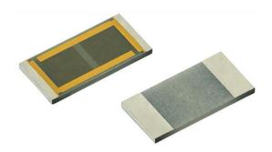
PCAN series chip resistors are designed on aluminum nitride ceramic substrates with enlarged backside terminations to reduce the thermal resistance between the topside resistor layer and the solder joint on the end users circuit assembly.
