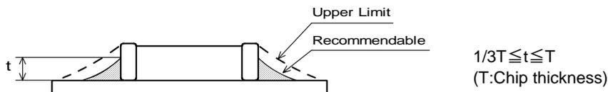
Accordingly increasing the solder volume, the mechanical stress to product is also increased. Exceeding solder volume may cause the failure of mechanical or electrical performance.
