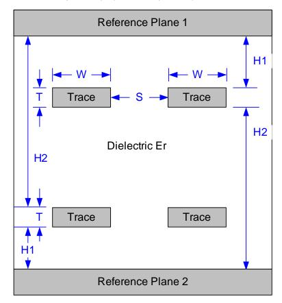
Figure 16. PCB Stacking Geometries
