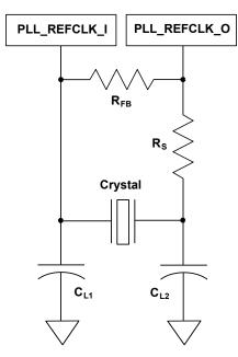
Figure 11. Recommended Crystal Oscillator Configuration
