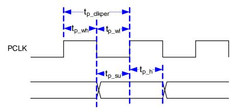
Figure 2. Parallel and BT.656 I/F General Timing
