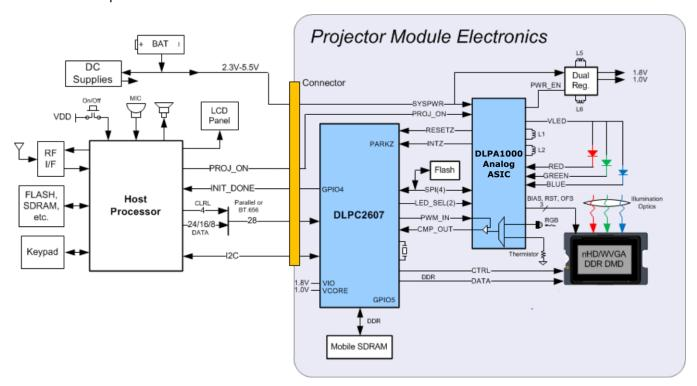
Figure 10. Typical Standalone Projector System Block Diagram
