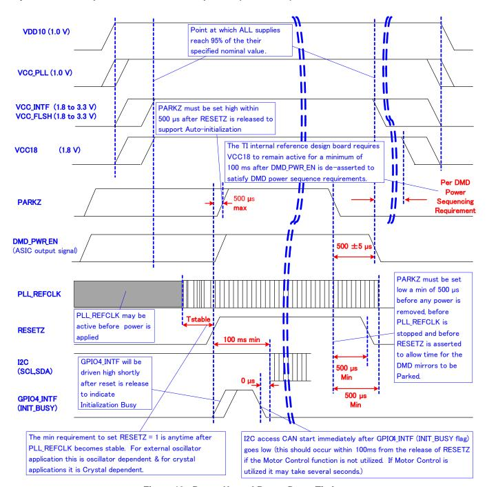
Figure 13. Power-Up and Power-Down Timing
