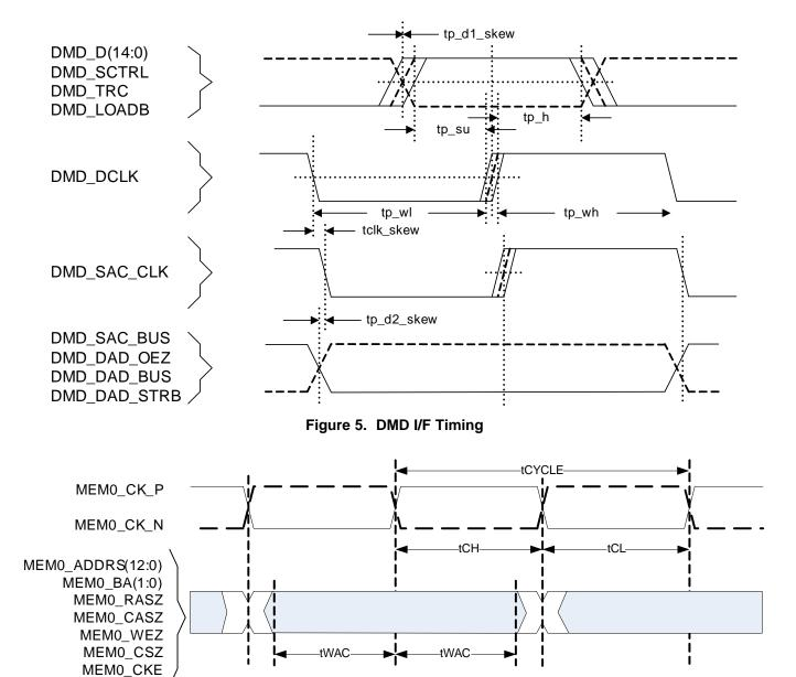
Figure 6. mDRR Memory Address and Control Timing
