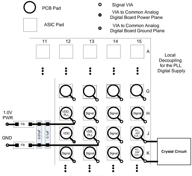
Figure 15. PLL Filter Layout
