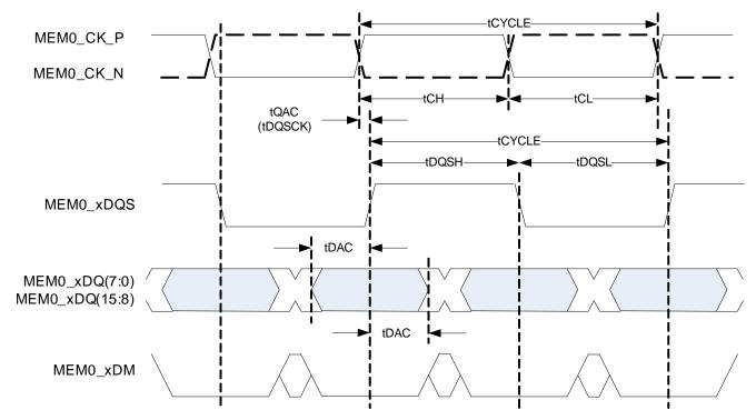
Figure 7. mDRR Memory Write Dtat Timing
