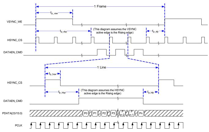
Figure 1. Parallel I/F Frame Timing
